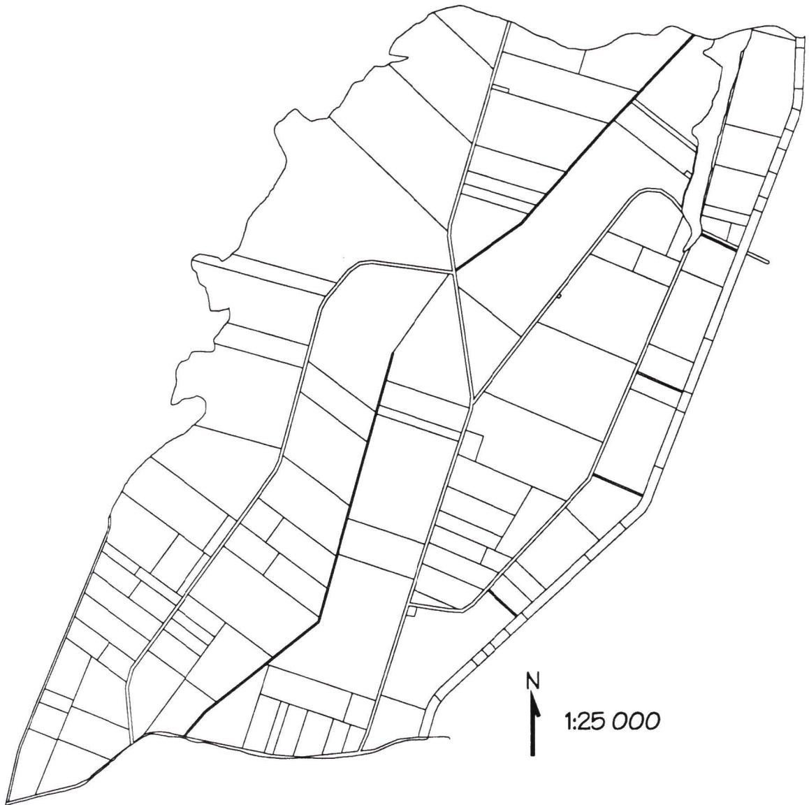
Figure 7.2 Cadastre after actual consolidation. Notice the new roads (double lines) and drainage ditch (single line parallel to right map boundary)
