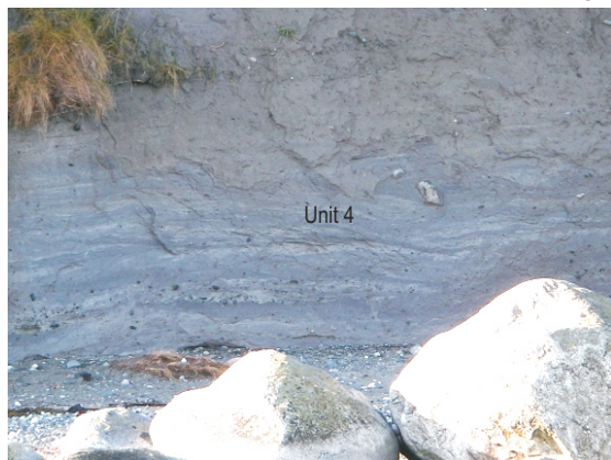
c) Lazo Bluff Section 9: 500 m along transect, GPS: 0365863, 5507235, vertical accuracy 6.7 m. Wavy to sub-horizontal bedding, pebble to boulder sized clasts.
