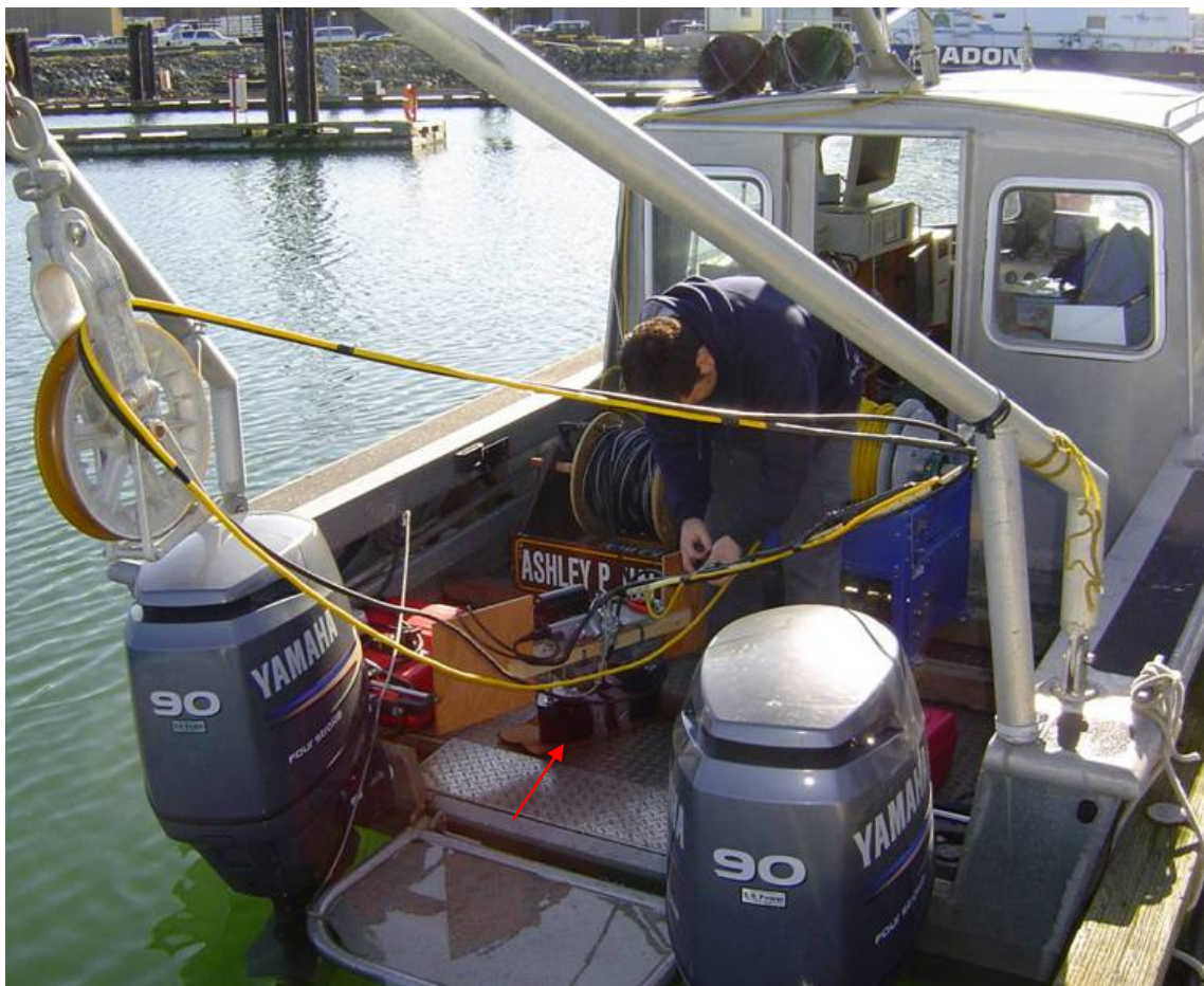
Figure 6-9. Apparatus setup aboard the CGR research boat for the depth dependence experiment. The red arrow points to the transducer. The ballast had not yet been attached. The apparatus was balanced in the water after adding ballast prior to deployment.
