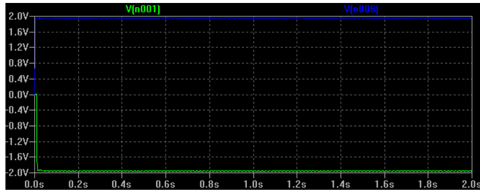
Figure 5.7: Output voltage of voltage doubler with active diode for 2.694V input, 1k \Omega load resistor.
