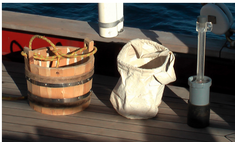
Figure 3.2: From left to right, the wood, canvas and rubber buckets used in the field comparison. Note that the wooden bucket was sealed with white caulk along the inner seams and reinforced around the outside by two stainless steel bands. The rubber bucket is of both plastic and rubber construction, with a black rubber protective layer around the base.
