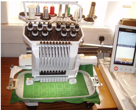
(a) Fabrication of a textile FSS using a digital embroidery machine [99].
