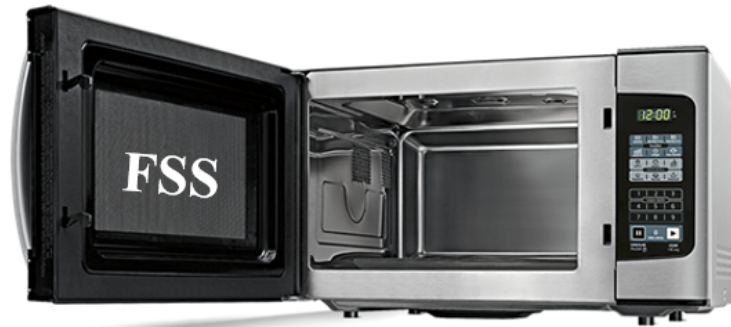
Figure 2.15: FSS embedded in the door of a microwave oven.
