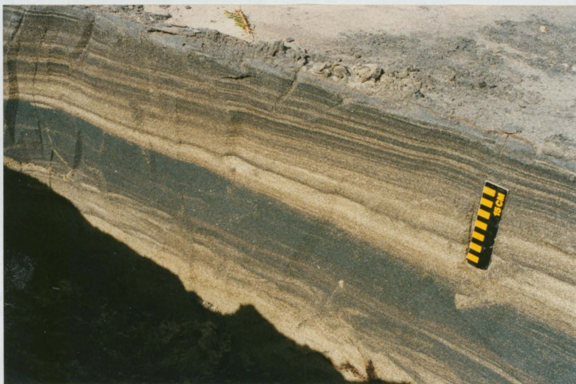
Plate 2. A trench within the study zone shows laminations of heavy and light minerals underlain by thick deposit of heavy minerals.
