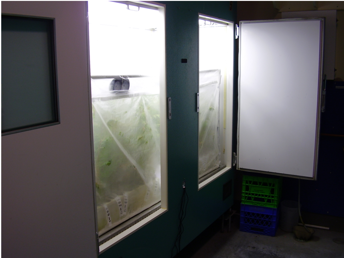
Figure A.1. Custom-made humidity chamber used to carry out controlled inoculations of Thuja plicata foliage with Didymascella thujina . The cage was made of PVC pipes fully covered with transparent plastic. An irrigation system linked to a tray inside the cage supplied the water used by five Exo Terra ® ultrasonic foggers (Rolf C. Hagen Inc., Montreal QC, Canada) to increase the relative humidity above 90% within two days. The excess water was drained by holes punched at the bottom of the cage. During the experiment, the cage remained inside a Conviron growth chamber (Conviron, Winnipeg MB, Canada) set at 12 h darkness at 10°C and 12 h light at 14°C. Temperature and humidity meters were placed inside the cage to monitor those conditions. (Image by Juan A. Aldana).
