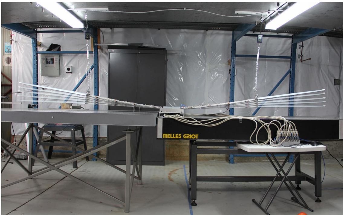
Figure 60: Single load point, symmetric static load testing of the wing.
