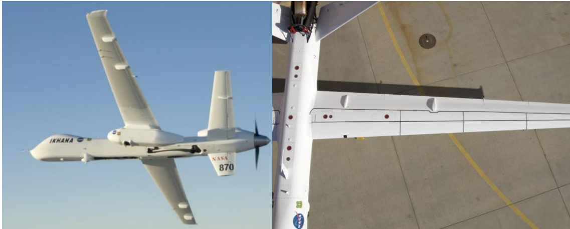
Figure 12: NASA Ikhana aircraft procured to support Earth Science missions and advanced technology development. Note in Left) black tape along upper wing surface concealing Fiber Optic Sensing System fibres for strain measurement[34].
