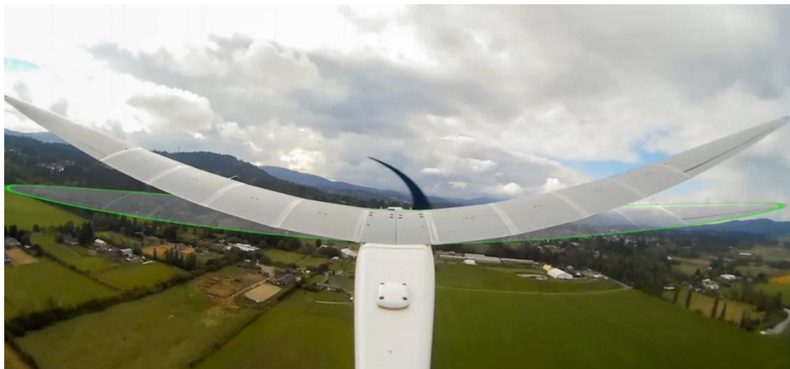
Figure 79: Flexible ASE QT1.3 flying over Saanich. Note wing shape while at rest on ground is traced in green overlay.
