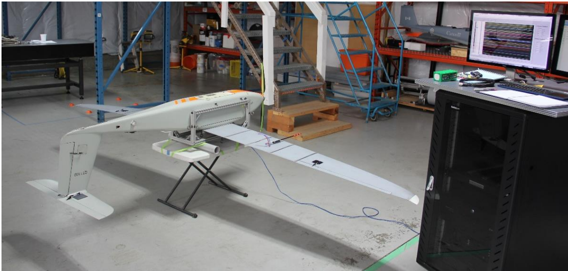
Figure 66: Strain compensation measurement to estimate wing droop following system tarring.
