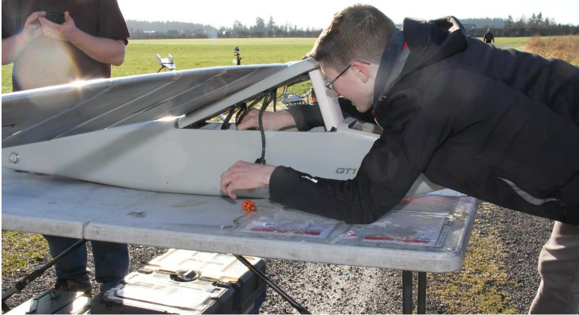
Figure 80: ASE QT1.3 undergoing pre flight assembly checklist. Individual strain gauge harness' are being installed.
