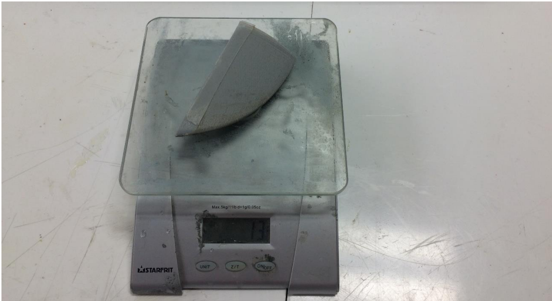
Figure 73: Winglet being weighed.
