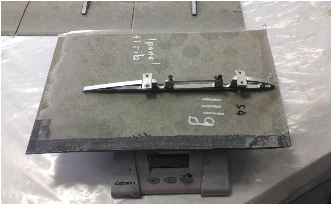
Figure 74: Mass of rib 4 and lower panel.
