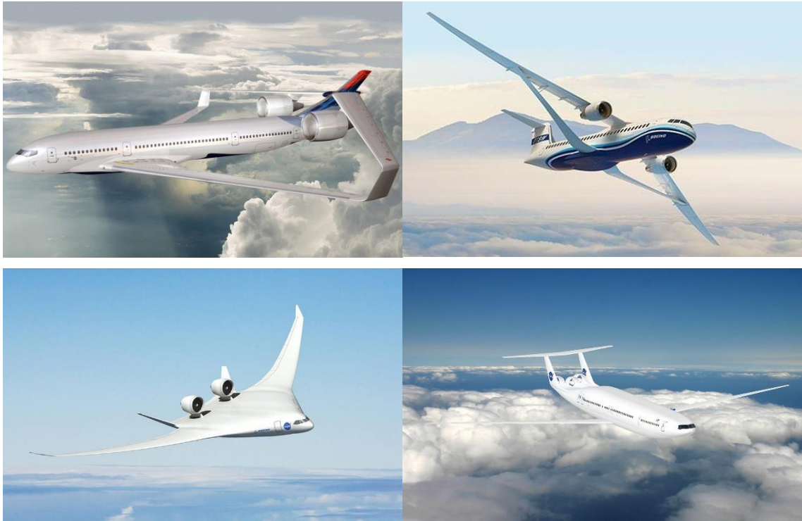
Figure 3: A joined wing concept from NASA and Lockheed Martin (Top Left) [13]. The Boeing SUGAR high aspect ratio truss braced wing (Top Right) [14]. The Boeing blended wing body concept aircraft (Bottom Left) [15]. The NASA, MIT, and Aurora flight sciences D8 concept aircraft with double fuselage configuration and high aspect ratio wings (Bottom Right).
