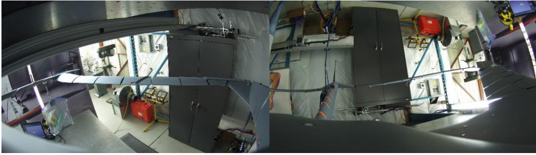
Figure 8: VMD tracking of bending and twist deformation of tail in CfAR flexible ASE JWSC project.
