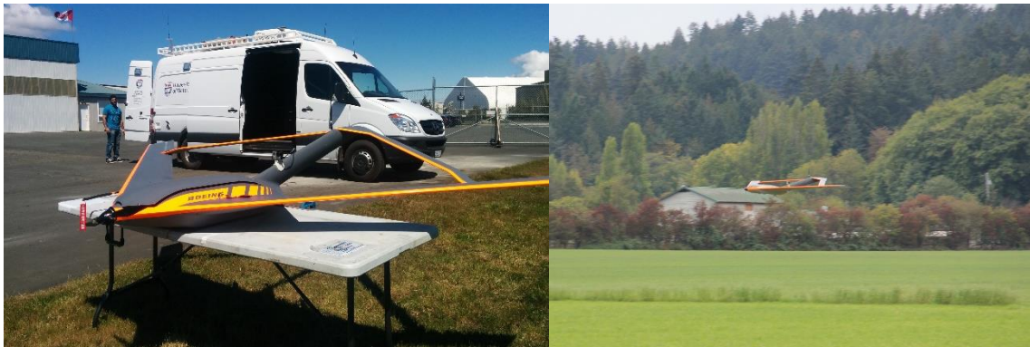
Figure 1: UVic CfAR 3m JWSC scaled flight test RPA
