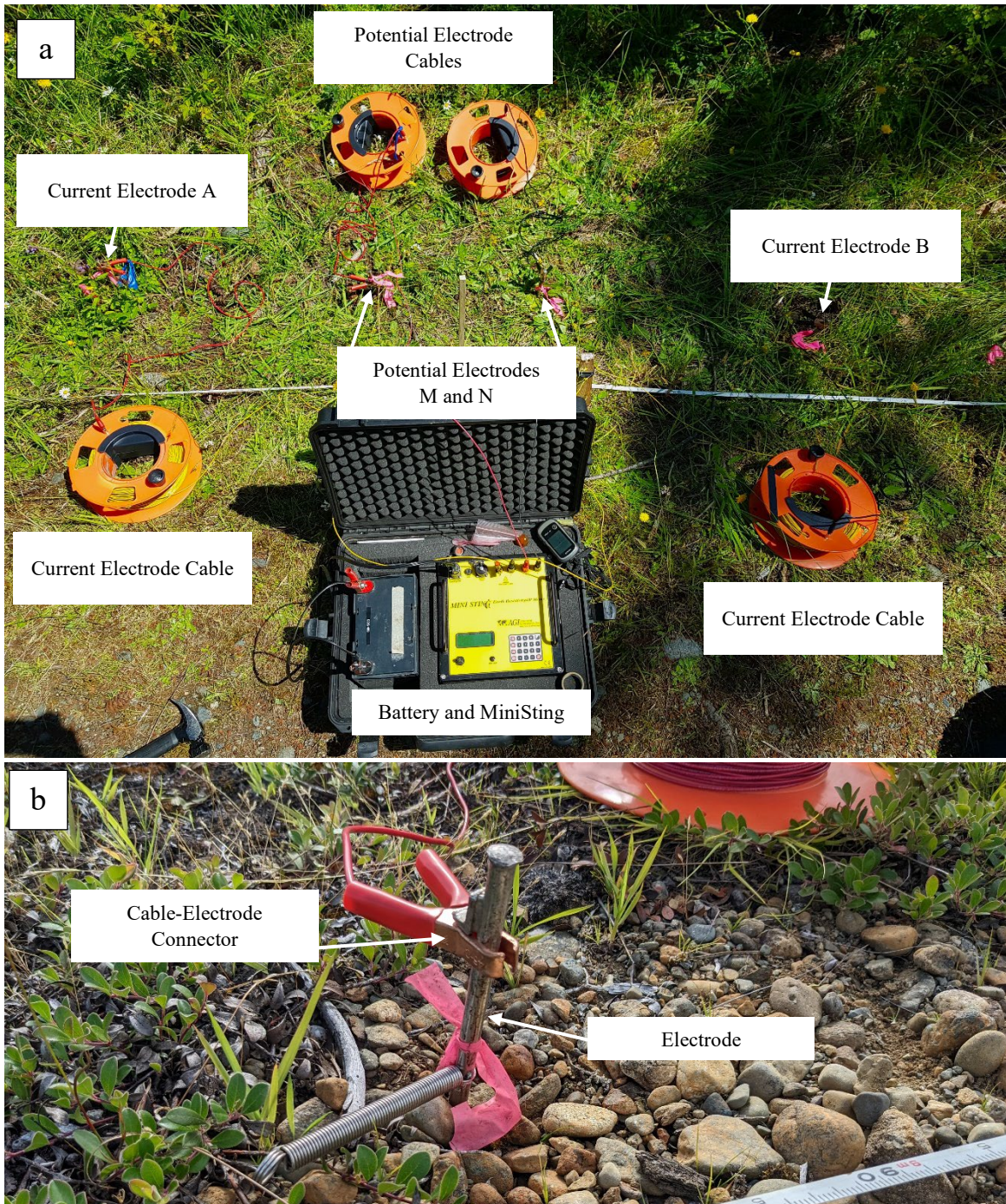
Figure 3.3.2. a) VES instrument setup showing all four electrodes, electrode cables, and the AGI MiniSting Resistivity Meter. b) Connection between electrode cable and potential electrode.
