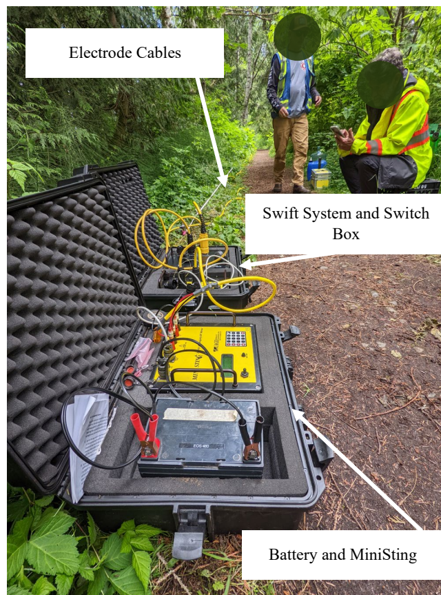
Figure 3.4.2.0. Equipment used in the ERT surveys. The foreground shows the battery connected to the AGI MiniSting Resistivity Meter, which is connected by cables to the Swift Automatic Multi Electrode System, and Switch Box in the middle ground. In the background, electrode cables are laid out and connected to the 28 electrodes along the left side of the dirt path.
