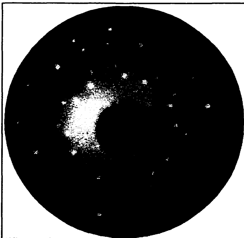
Figure 4.6- (\sqrt{7}\times\sqrt{7})R19.1^\circ -I LEED Pattern (100 eV)
