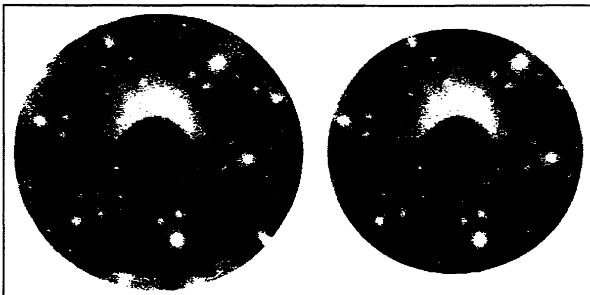
Figure 3.9-Removal of Ring Due to Fringe-Field Plate (Photo Taken at 135 eV)
