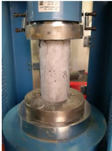
Figure 7 Compression test on Forney machine
