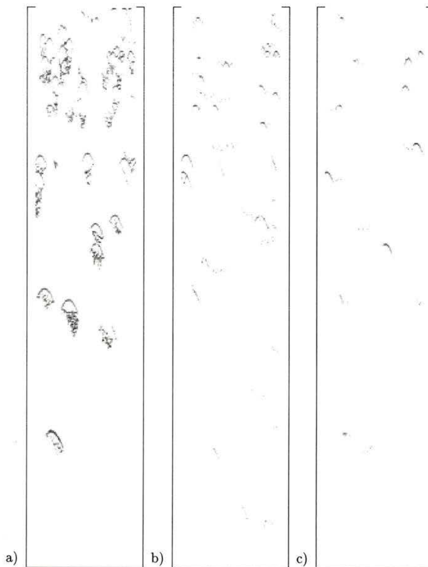
Figure 3.11: The particle tracks found in image S2. The Streaks classification used the results of the a) dPeak, b) Deconv-dPeak, and c) Wavelet-dPeak algorithms.
