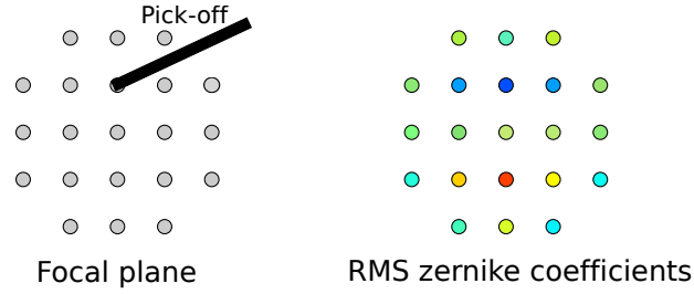
Figure 1.6: Field dependent aberrations in the field of view of a telescope. When changing the pick-off position in the focal plane (left), the field dependent aberration seen depends on that position (right).
