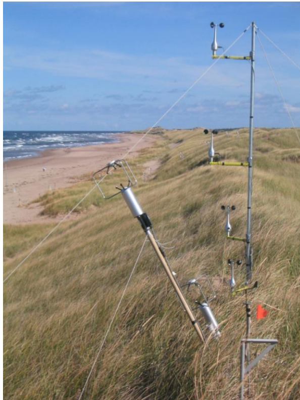
Figure 2.5: Photographs of the study site. (a) The transect ran from the toe of the dune to the crest and had a total of four different locations with six stations. (b) The stations were located at two different heights, 1.66 m and 0.60 m, and were aligned with the underlying surface slope.
