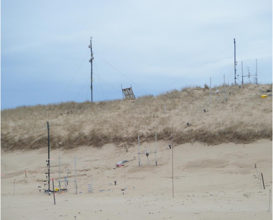
Figure 3.5: Photograph of the study site. The transect ran from the beach to the crest of the dune and had a total of four different locations. The 3-D sonic anemometer stations at the beach and crest were located at two different heights, 1.2 m and 0.2 m, whereas, the 3-D sonic anemometer stations at the toe and the stoss were located at a height of 0.2 m. All stations were aligned with the underlying surface slope and each location had a co-located Wenglor Laser Particle counter at 1.4 cm.
