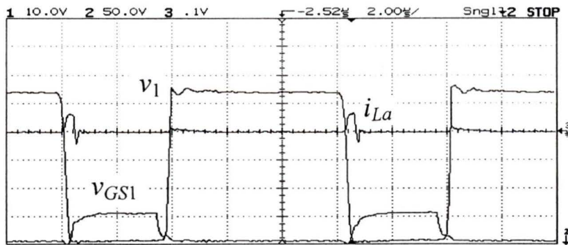
The auxiliary inductor current, i_{La} (2 A/div), (iii) Gate-Source voltage, v_{GS1} (10 V/div) and switch S1 voltage, v_1 (50 V/div)
