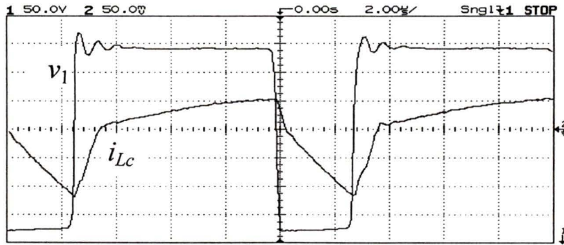
(i) dc-to-dc section inductor current, i_{Lc} (5 A/div) and switch S1 voltage, v_1 (50 V/div)
