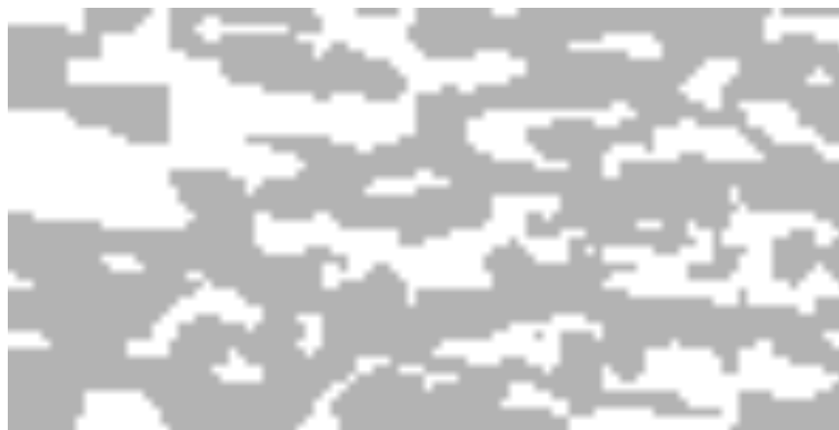
Figure 4.2: One of the slices in the x-y plane of the catalyst layer of dimensions 1 \mu\text{m} \times 1.98 \mu\text{m} \times 1 \mu\text{m} . The white represents the gas and the grey represents the solid with no distinction between the carbon and ionomer.
