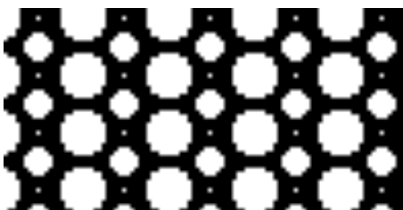
Figure 5.4: Slice of the idealized CL of dimensions 1\ \mu\text{m} \times 1.98\ \mu\text{m} \times 1\ \mu\text{m} with no perforations. The solid and gas are represented by white and black respectively.
