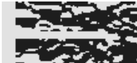
Figure 5.3: Slice of the reconstructed geometry with a perforation 1.5\mu\text{m} in length along the y axis.
