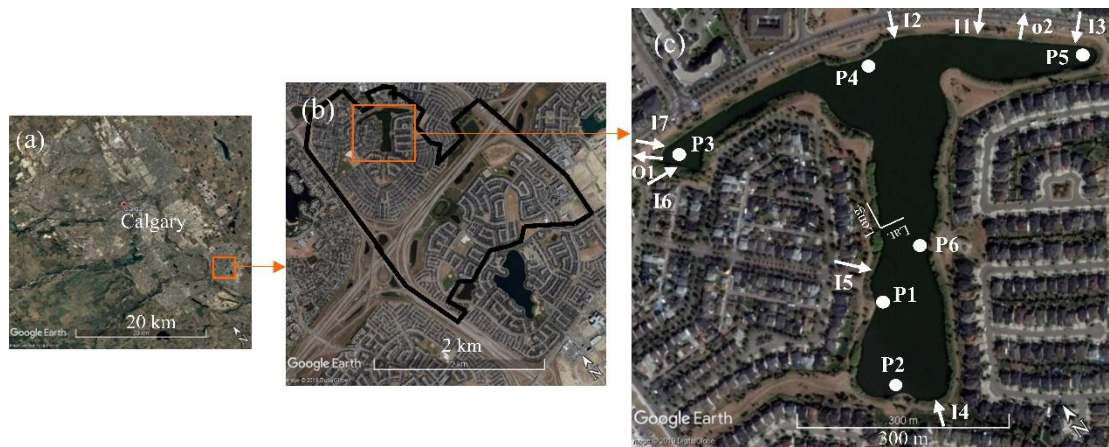
Figure 3.1 The study site: (a) aerial view of the City of Calgary; (b) the catchment of the Inverness Stormwater Pond (the dark solid line – catchment boundary); and (c) the locations of inlets (I1~I7), outlets (O1 and O2), and sampling locations (P1~P6) in Inverness pond [50°54'39.55"N 113°57'48.4"W at the centre of the map]
