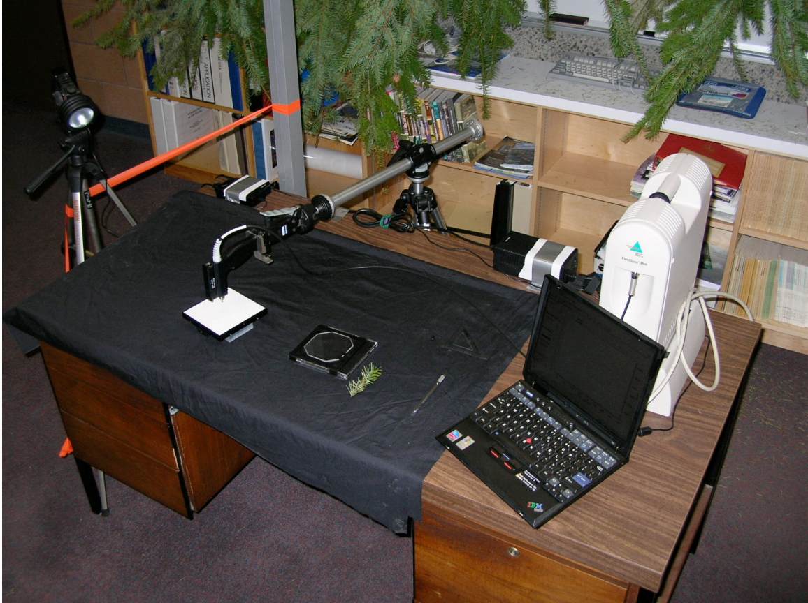
Figure 3-6: Instrumentation layout for reflectance measurements.
