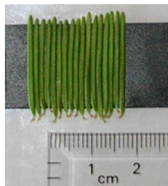
Figure 3-5: Douglas-fir needles prepared for spectral reflectance measurement.
