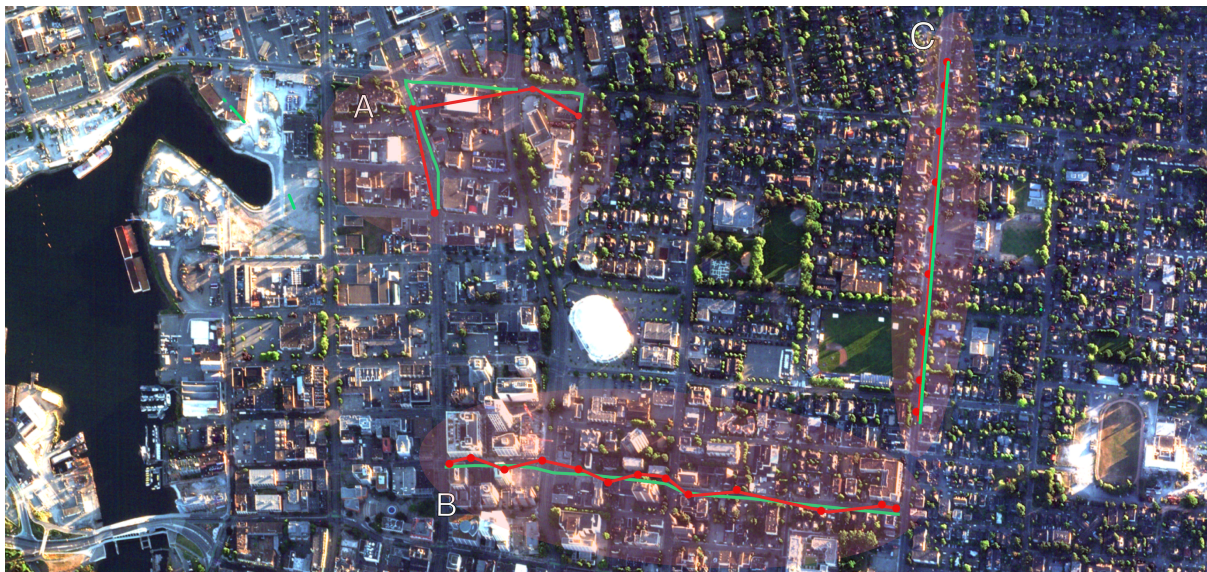
Figure 4.1: An illustration of GPS errors. Green represents ground truth and red represents trajectories created by connecting recorded real-time bus positions
