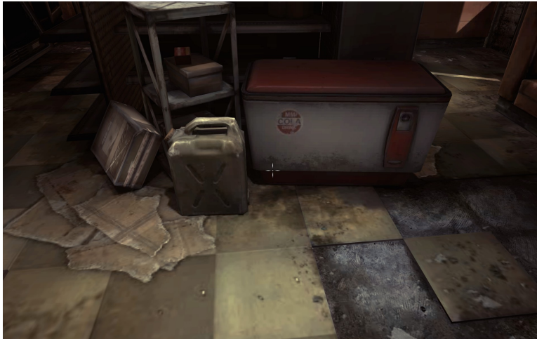
Figure 2.3.2: An area of poor texture quality in RAGE. Also note the artifact on the floor caused by incorrect bilinear filtering across a page boundary in the virtual texture. Image (C) id Software.
