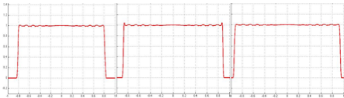
Figure C.6: The output of a 16-band 3D QM-CM cone filter for the first thirteen discs, the first fourteen discs, and the first fifteen discs
