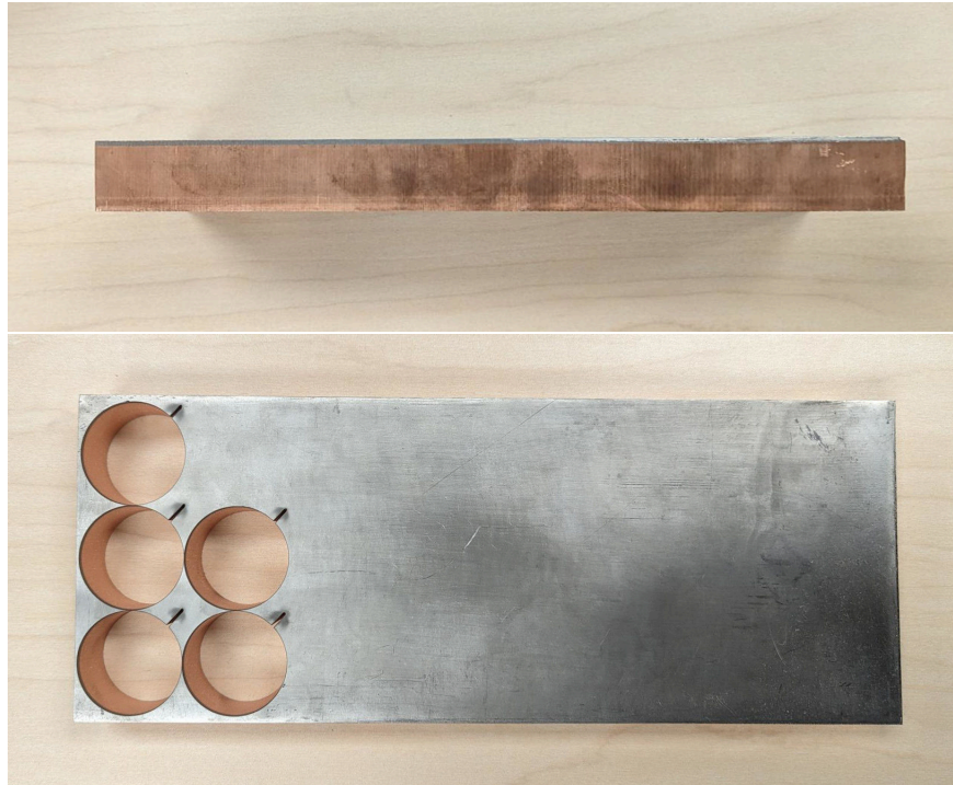
Figure 3.10: Explosion bonded block viewed from the side (above) and top (below).
