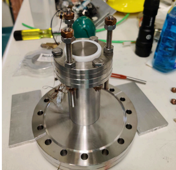
Figure 3.16: Assembled sample spool with (left) and without (right) the PTFE calibration block.
