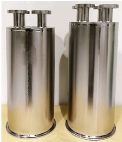
Figure 2.6: Quarter-wave (left) and half-wave (right) resonator test cavities from TRIUMF's coaxial program.
