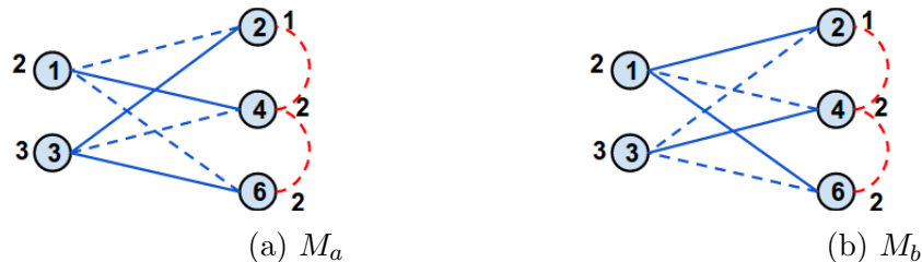
Figure 3.12: An example illustrating the difficulty in determining when to stop the algorithm if there exists a PAP. Solid blue lines represent the current matching M . Dashed blue lines are unmatched edges. Red dashed lines on the right side are conflict constraints between buyer nodes.
