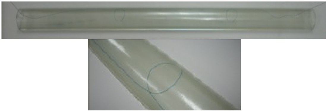
Figure 3.7: Semicircular tube with embedded fiber optic sensors
