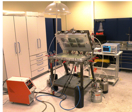
Fig. 1 Schematic of RTM process (left) and the lab apparatus including optical equipment (right)
