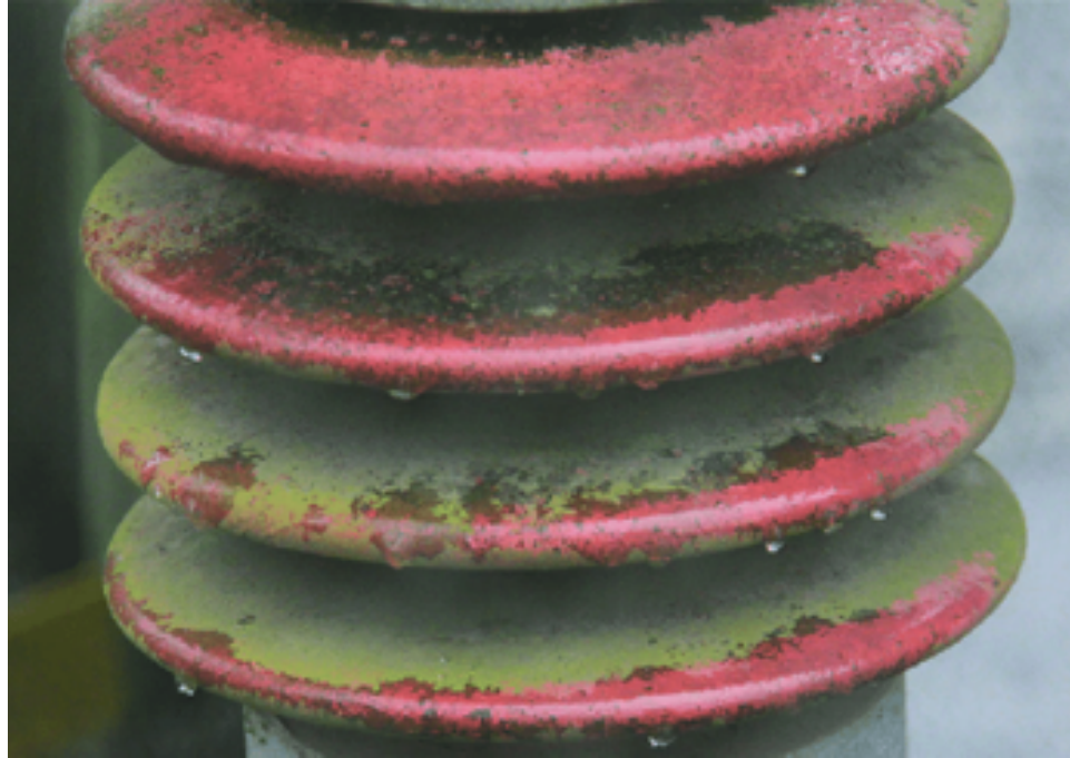
Figure 1.2: Illustration of the microalgae biofilm on the electrical insulator [7].
