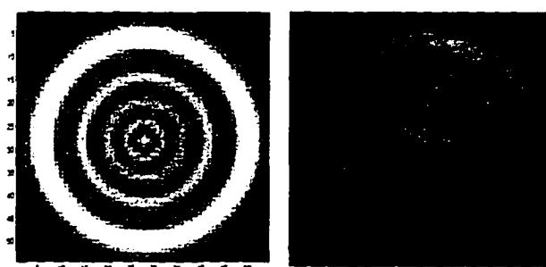
Figure 2.32 Defocused PSF for the 40x, 0.65NA lens at the defocus amount of 10\mu\text{m} . Left: theoretical result; size: 54 \times 54 . Right: experimental result; size: 41 \times 41 .
