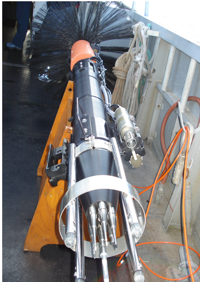
Figure 2.3. The Vertical Microstructure Profiler on the deck prior to profiling. The CTD unit is visible on the right side. The temperature and shear microstructure sensors are visible at the bottom of the image.
