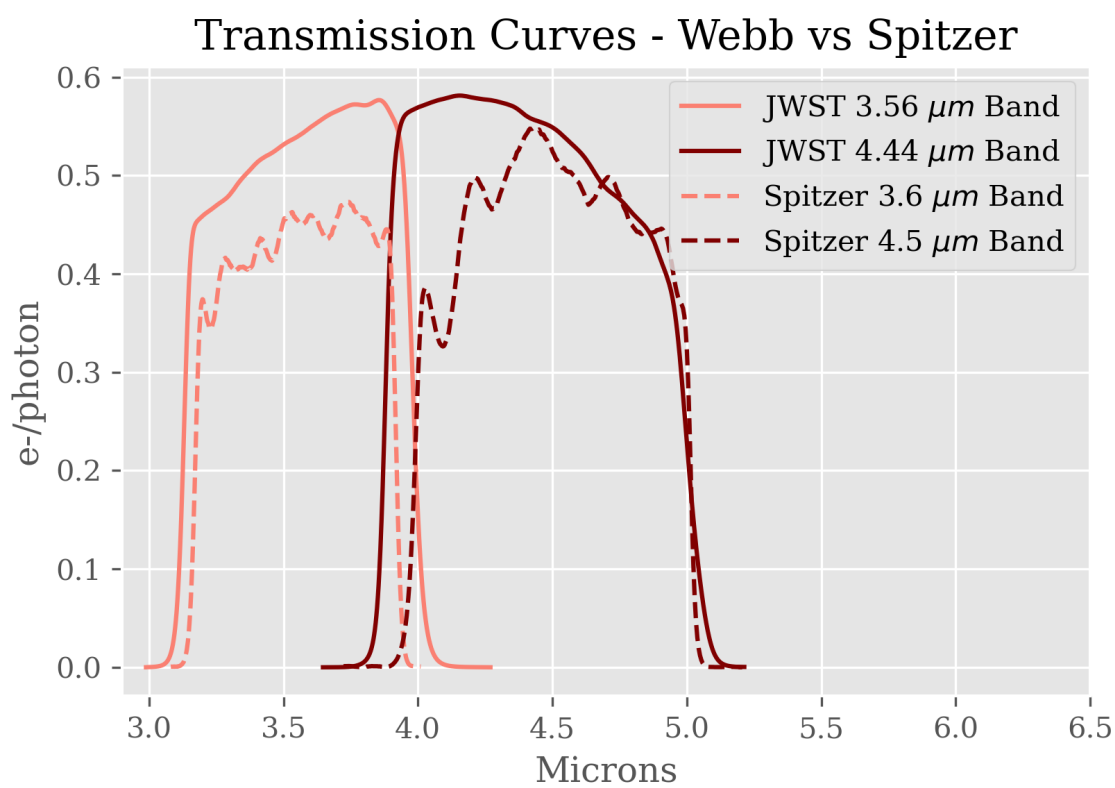
Figure 1.3: Transmission curves of both JWST (solid lines) and Spitzer (dashed lines) for the JWST NIRCам bands that match the Spitzer bands. JWST has an additional 27 filters in NIRCам that are not shown in this comparison.
