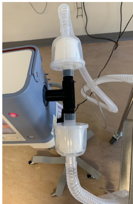
Figure 3. A 3D printed T-Piece Ventilator Splitter connected to a ventilator. This image is reprinted under a Creative Commons Attribution 4.0 International License and it is from [50].
