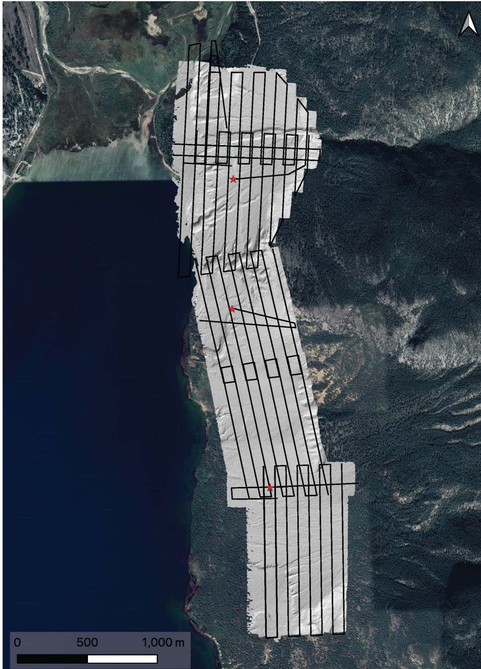
Figure B.4: Flightlines for the Southern Rocky Mountain Trench site. Black lines are flight lines superimposed on the resultant DTM. Red star indicates the takeoff and landing location for the collection. Satellite imagery from Google.
