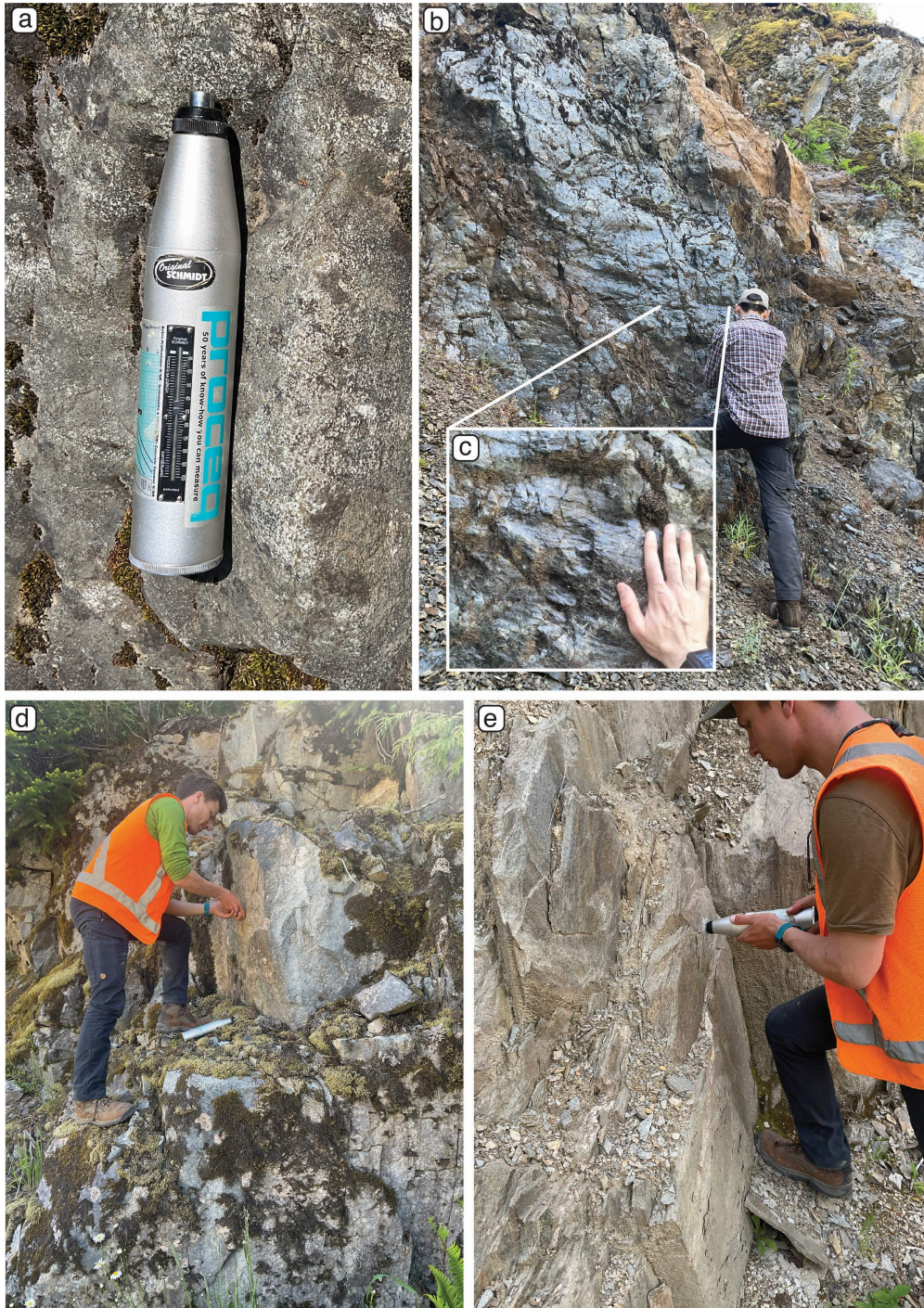
Figure C.19: Photographs from the Schmidt hammer data collection. a) Proceq N-type Schmidt hammer used for data collection. b) Sub-vertical fault shear zone located near the uphill facing scarp. c) Close-up of the serpentinized material. Some near-horizontal slickenlines present. d) Cleaning the surface for Schmidt hammer sampling. e) Taking a sample, most samples were collected from near vertical surfaces along roadsides.
