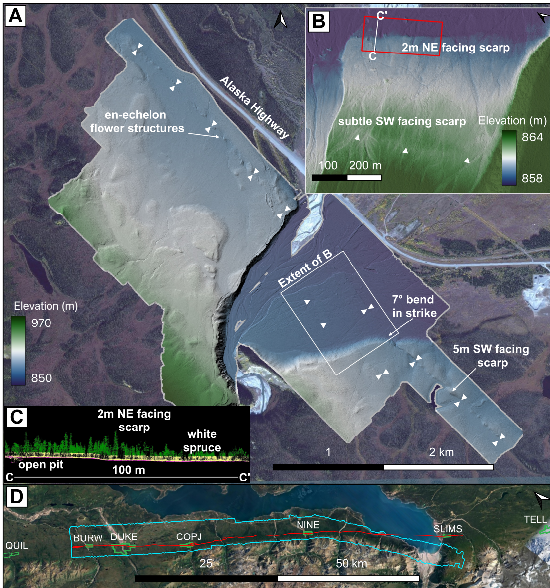
Figure 3.11: (A) Hillshaded drone lidar DTM of the Duke River site on the Eastern Denali fault (EDF). The extent of panel B is marked by the white rectangle. White triangles indicate the approximate location of the EDF. Underlying satellite imagery is from Bing. (B) Inset showing a 2 m high northeast facing scarp along a river terrace. The red polygon shows the bounds of the flight parameter testing discussed in Section 3.10.1. White line shows the location of cross section C–C'. (C) Cross section C–C' through the classified ULS point cloud, with green for vegetation, pink for ground returns, and yellow for unclassified points. (D) Locations of all ULS collection sites (green polygons) along the trace of the EDF as identified with lidar data (red line). The cyan polygon outlines the comparison ALS dataset. Satellite imagery is from Google. QUIL = Quill Creek, BURW = Burwash Creek, DUKE = Duke River, COPJ = Copper Joe Creek, NINE = Nines Creek, SLIMS = Slims River/Topham Creek, TELL = Telluride Creek.
