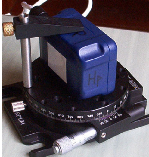
Figure 4.3 Magnetic compensation testing set-up for Xsens MT9 IMU.
