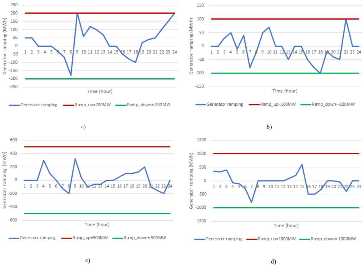
Figure 2: Ramping values of four arbitrary generators over 24 hours; a) generator 1, b) generator 2, c) generator 3, d) generator 4
