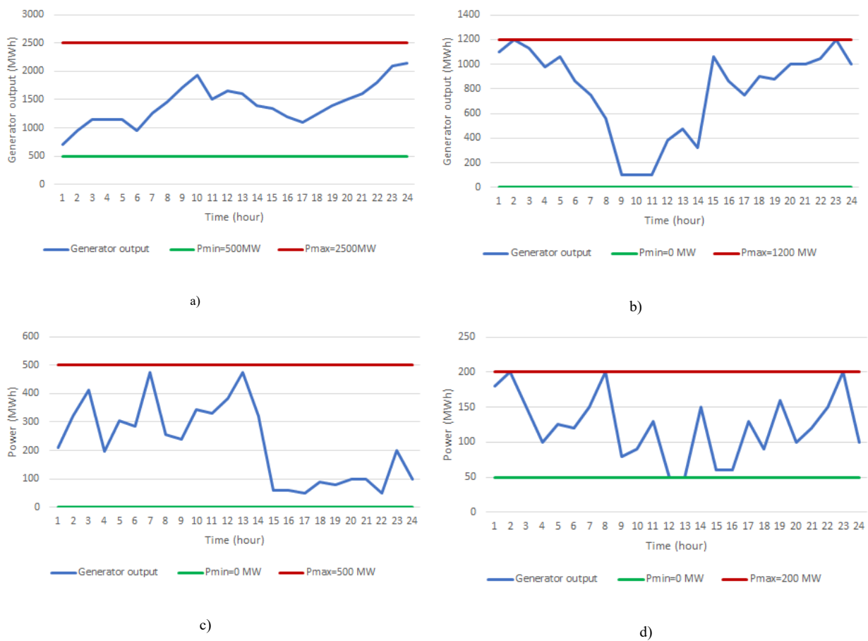
Figure 1: Output power of four arbitrary generators over 24 hours; generator 1, b) generator 2, c) generator 3, d) generator 4
