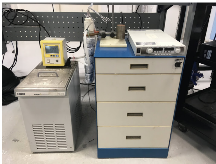
Figure 5.1: Experimental setup (From left to right – LAUDA E20 cooling bath, thermosyphon for testing, and power source)
