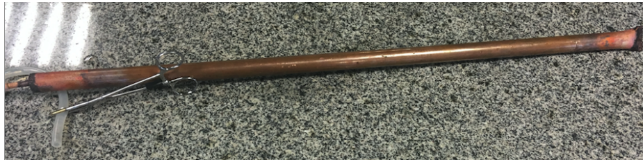
Figure 4.5: Example of thermosyphon with umbilical tube in one end and clamped in the other end
