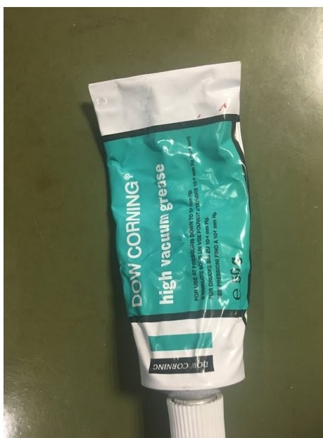
Figure 4.10: High vacuum grease used for sealing
