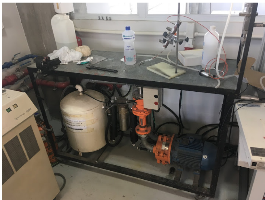
Figure 4.7: Roughing vacuum pump in the lab
