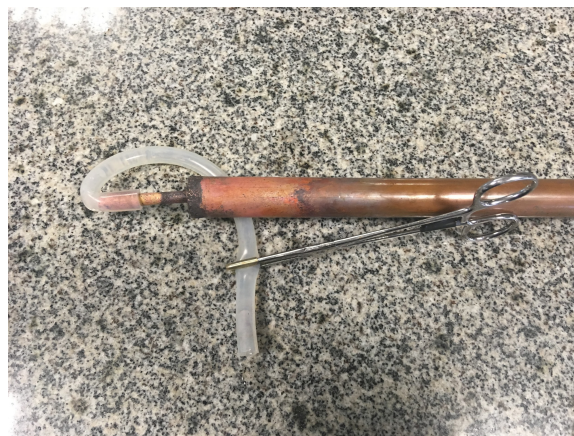
Figure 4.2: Umbilical tube and lid welded in one of the thermosyphon's ending
