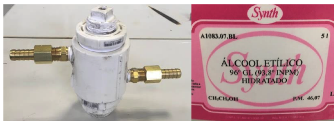
Figure 5.2: Sleeve for the condenser section to allow liquid circulation (left). Ethyl alcohol used inside the cooling bath (right).
