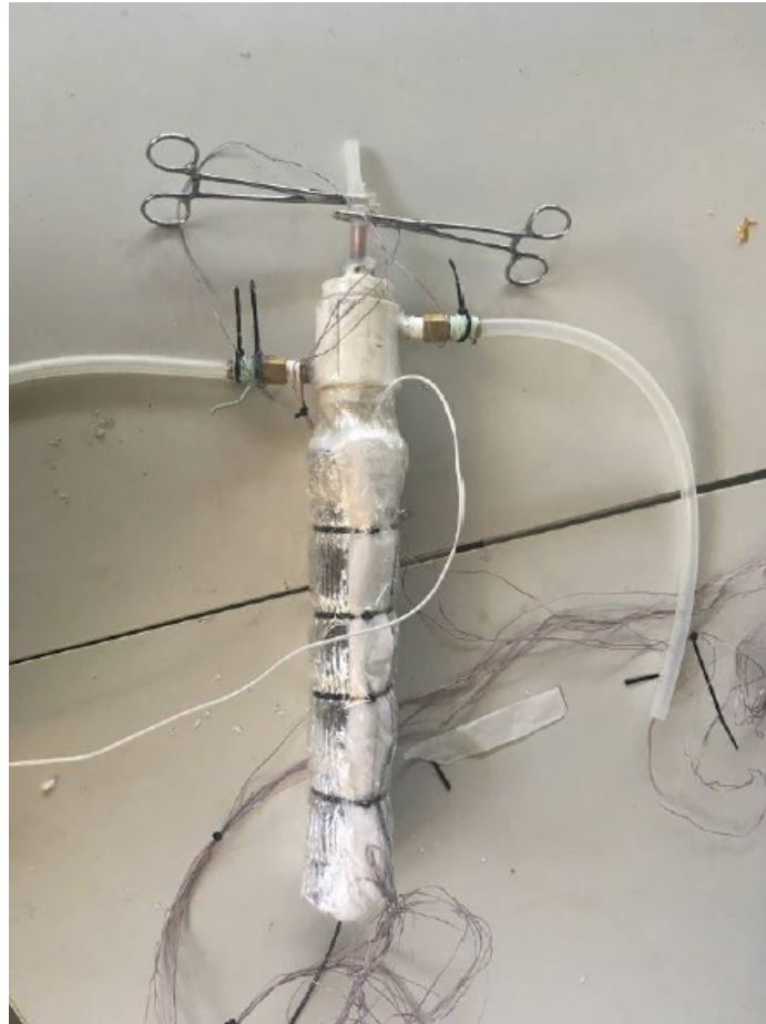
Figure 5.4: Thermosyphon insulated, instrumented and ready for experimental testing
