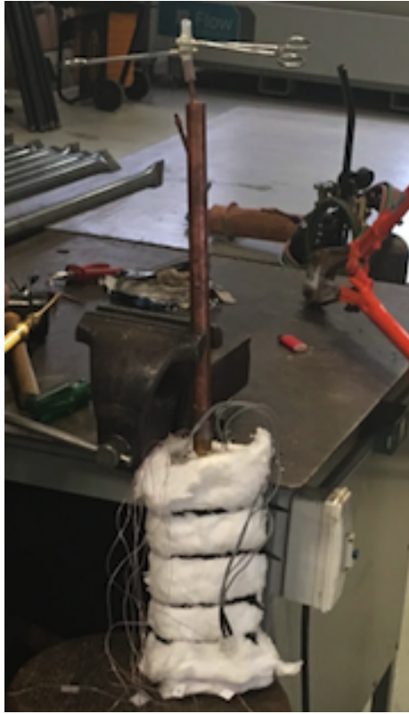
Figure 4.13: Sealing procedure in order to close the thermosyphon completely.
