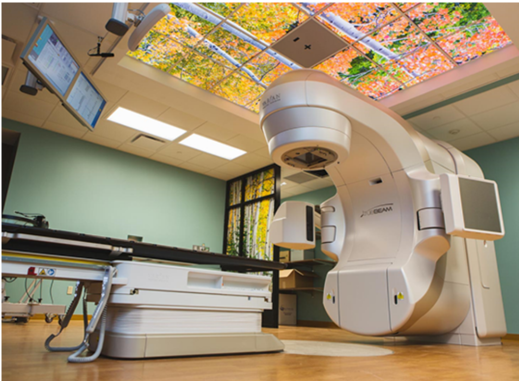
Figure 1.1: A Varian TrueBeam linear accelerator (Palo Alto, California, USA) which is used to treat patients with megavoltage electron and x-ray beams. [7]
