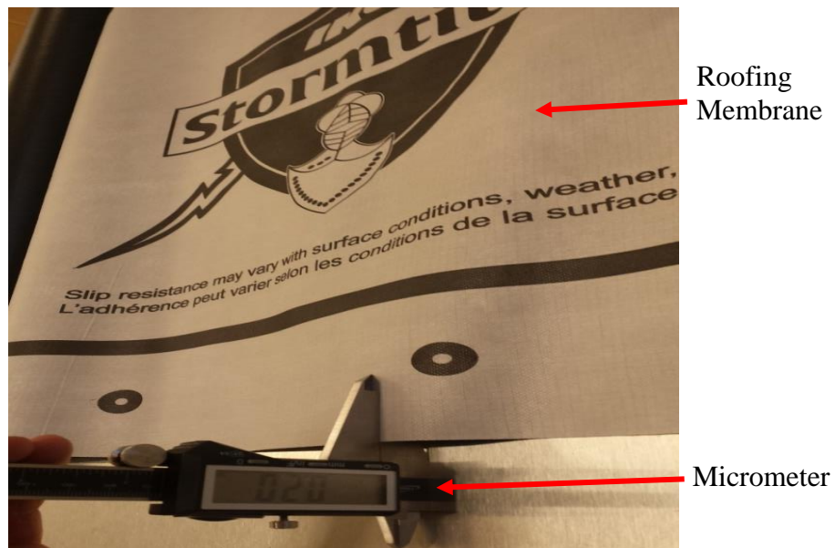
Figure 7 - Measuring the thickness of roofing membrane using Vernier caliper
