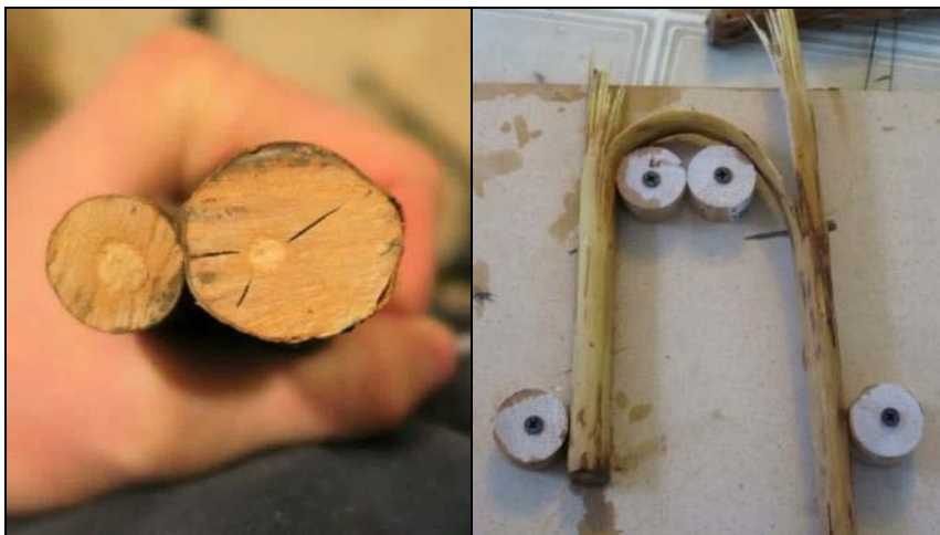
Figure 33: Left image showing oceanspray with different pith thicknesses. Right image showing failed steam-bending attempt.
