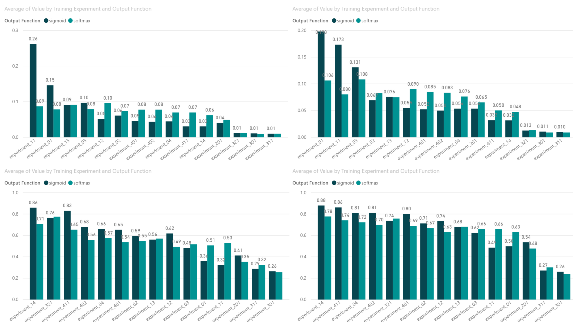
Figure 7.17: Recall and precision comparison between output functions from most experiments' models on human and mouse chromosome data
