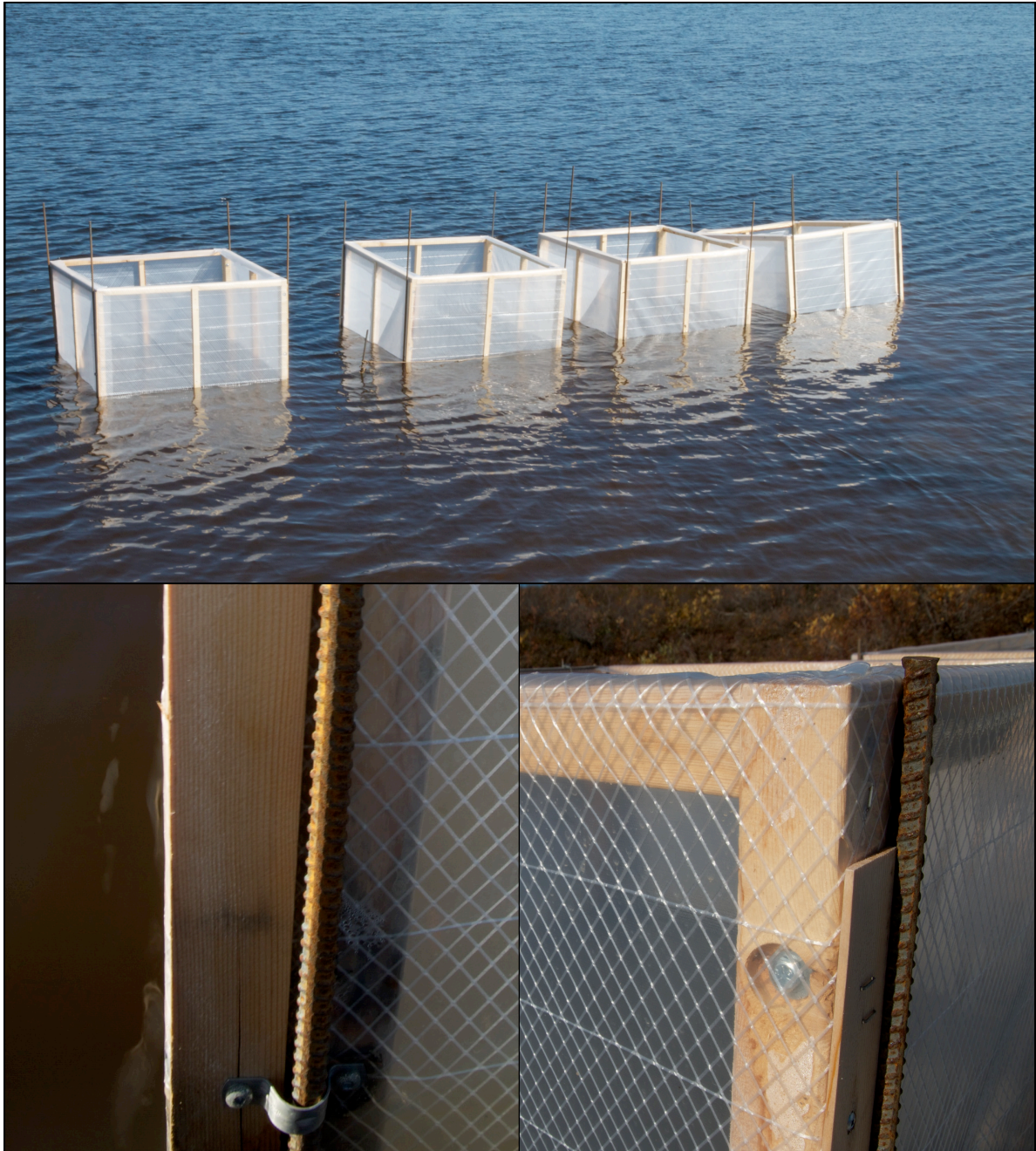
Figure A.3. Top: Four 8-foot pieces of rebar, one in each corner are used to affix the mesocosms to the lake floor. Bottom left: Rebar treaded through two aligned “U” brackets. Bottom right: Rebar is pounded with a sledgehammer until flush with top of the mesocosm. Note use of recessed washer and bolt as well as wood lathing to prevent the plastic sheeting from moving.
