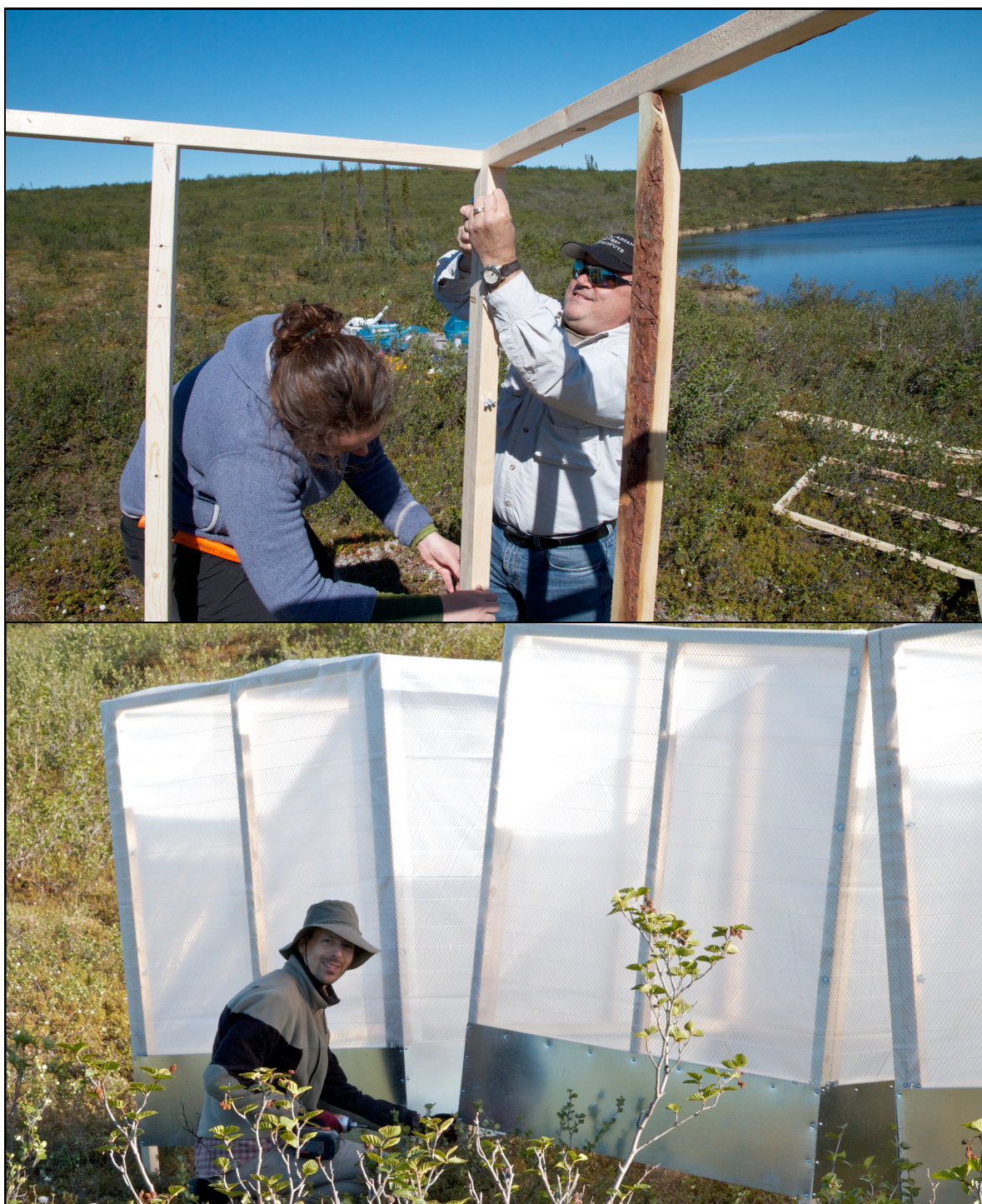
Figure A.2. Top and bottom: Assembly of mesocosms before installation.
