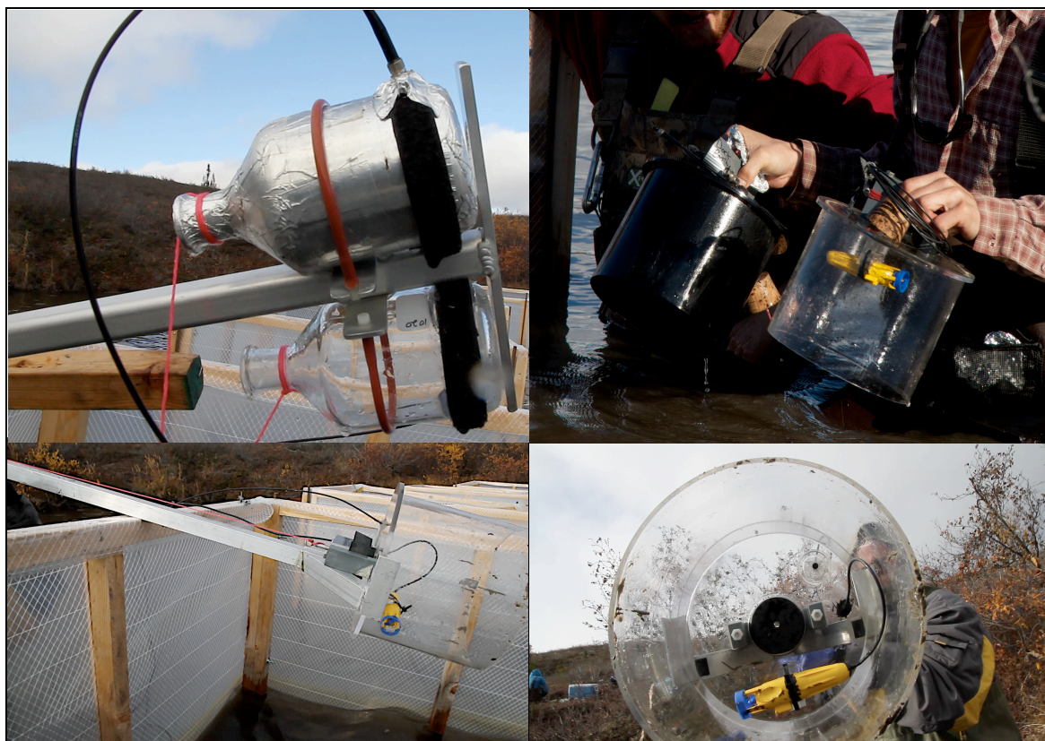
Figure 4.2. Light and Dark bottles with fibre optic cables protruding (top left). Light and dark benthic samplers (top right and bottom). Samplers were pushed into the sediment with the aluminum pole. A spring-loaded stopper was kept open during installation and was closed thereafter. A small (yellow) motor circulated the water just prior to reading.
