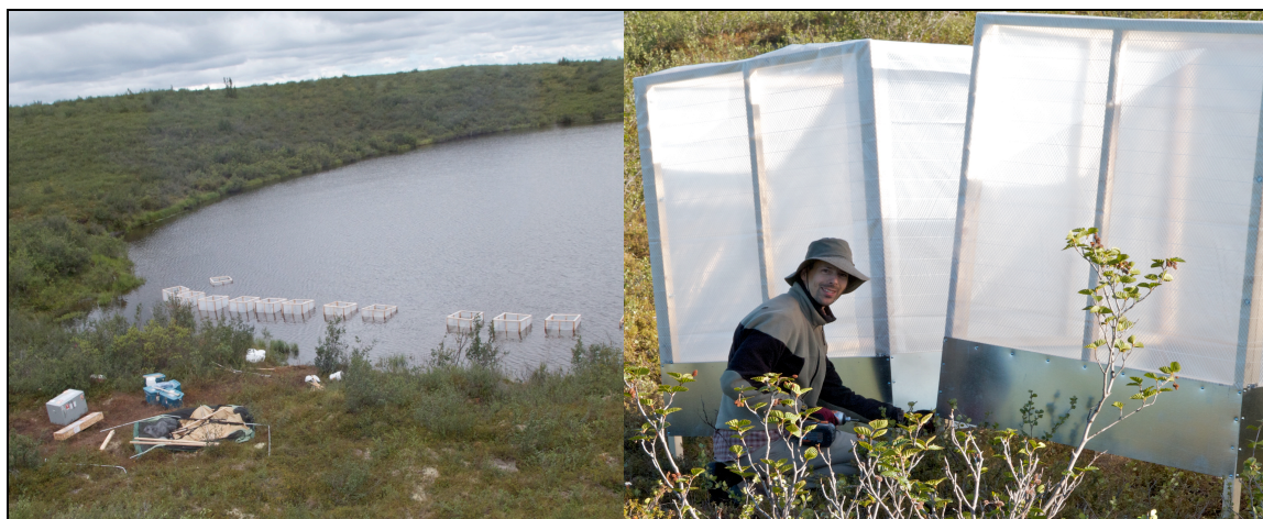
Figure 2.3. Left: Mesocosms set up at 1 meter depth of Lake 5A, a typical tundra lake on the uplands of the Mackenzie Delta. Right: Mesocosm assembly prior to installation.
