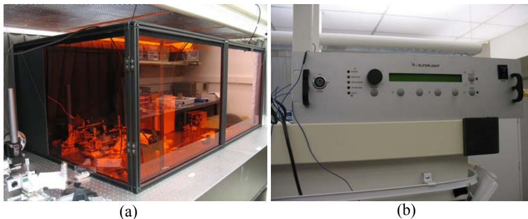
Figure 4.4. Laser protective enclosure and laser head control panel
