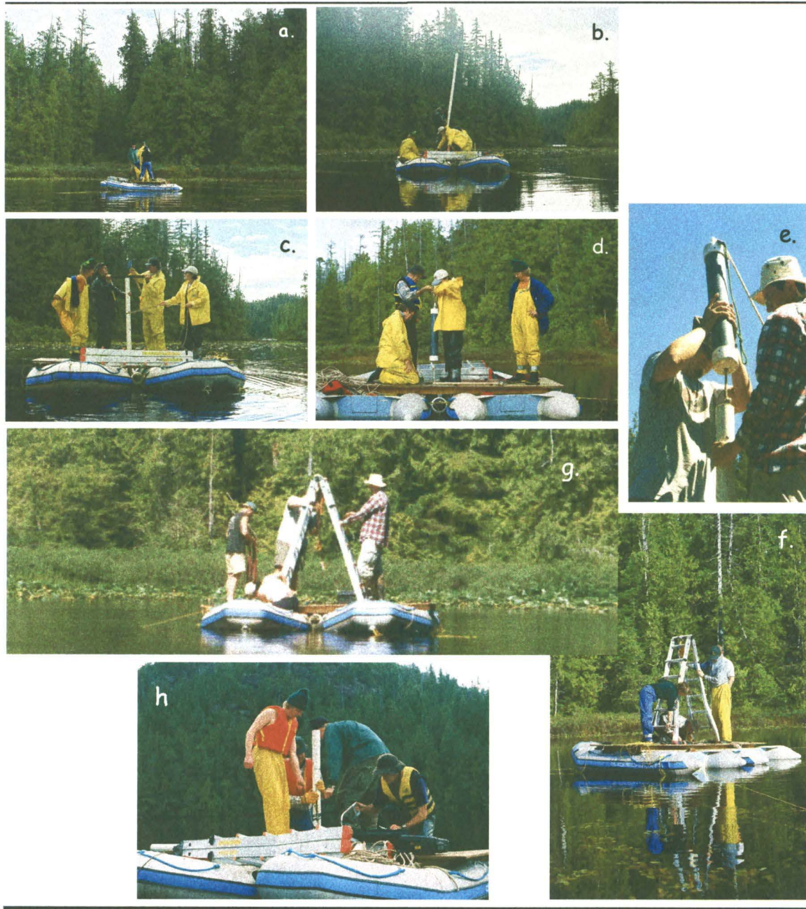
Figure 2.7 Sequence of photographs illustrating the percussion coring technique used in this research: (a) Stabilizing the coring platform with anchors on the four corners; (b) Introducing the first PVC pipe into the waters and surficial sediments of the lake bottom; (c) The initial percussion coring is carefully achieved with a sledge hammer until the pipe structure is at an accessible height to use the cement hammer shown in (d) and (e); (f) and (g) show the initial retrieval of the sediment core with a winch hooked to a step ladder, after coring is complete. Once the sediment core is released from the entrapping lake sediments, manual retrieval is possible (h), and subsequent cutting is performed. (Photographs taken at Kakawis Lake during field seasons 1998 and 1999).
