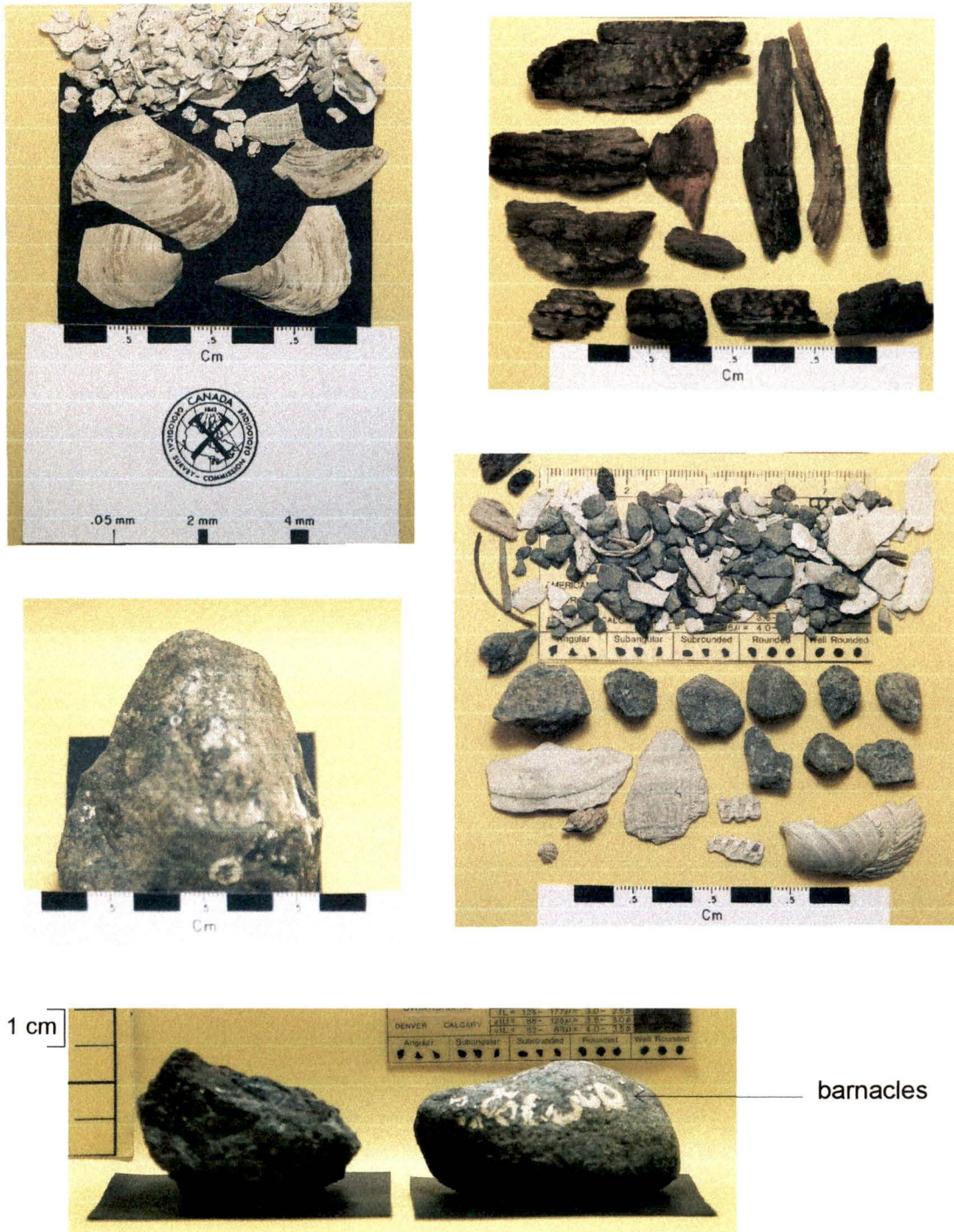
Figure 3.9 Examples of terrigenous, vegetation and carbonate material found in different tsunami facies of cores recovered from Kakawis Lake. Coarser clasts often showed fossil marks of barnacles (typical intertidal crustacean species). The particles shown here are part of the macro- (>2mm) elemental fraction forming any given tsunami event at this particular lake.
