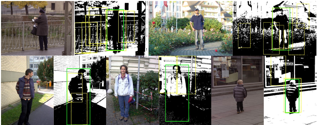
Figure 6.2: Examples of the INRIA person dataset include one person in RGB and binary format. Green and yellow rectangles show detection bounding boxes according to the ground truth dataset and detection results of our binary dual-feature system, respectively. False positive and false negative rates are not zero in these examples. The RGB format of images is only shown to represent details that are not clear in the binary format.
