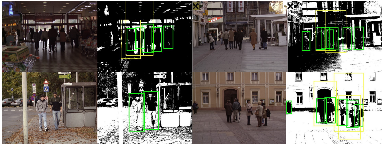
Figure 6.3: Examples of the INRIA person dataset include more than one person in RGB and binary format. Green and yellow rectangles show detection bounding boxes according to the ground truth dataset and detection results of our binary dual-feature system, respectively. The RGB format of images is only shown to represent details that are not clear in the binary format.
