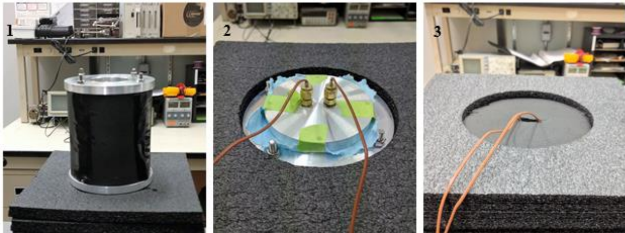
FIGURE 36: ADDING ADDITIONAL INSULATION TO THE TESTING APPARATUS AROUND THE HEAT SINK AND UPPER SEALING PLATE.
