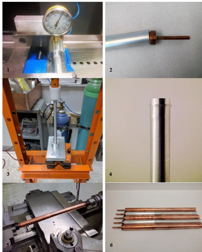
FIGURE 31: VARIOUS PRESS FITTING METHODS. ON THE LEFT ARE THREE DIFFERENT DEVICES USED TO PERFORM THE PRESSFIT; 1. A VICE, 3. A HYDRAULIC PRESS AND 5. A LATHE. ON THE RIGHT THE RESULTING PROBLEMS WITH THE FIRST TWO METHODS, 2. AND 4. AND THE FINAL ASSEMBLED 2 ND GENERATION BETA PROTOTYPES AT 6.
