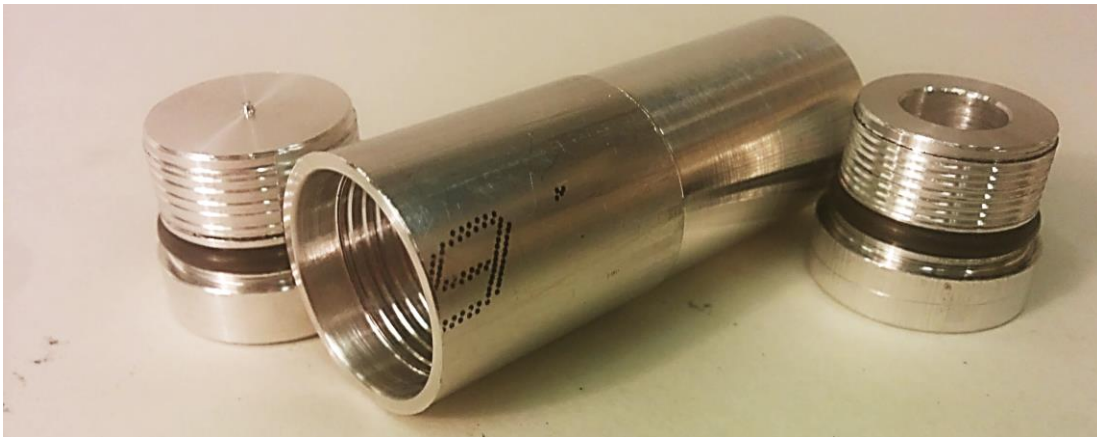
FIGURE 29: PROTOTYPE HEAT PIPE USED FOR PRESSURE TESTING. THE ENDCAP ON THE LEFT IS BARBED WITH AN O-RING TO CREATE A FLUID SEAL, THE BODY IN THE MIDDLE IS BARBED ON THE INSIDE TO INTERFERE WITH THE ENDCAP AND LASTLY THE ENDCAP ON THE RIGHT HAS AN NPT FEMALE THREAD TO CONNECT COMPRESSED AIR AFTER THE HEAT PIPE IS ASSEMBLED.
