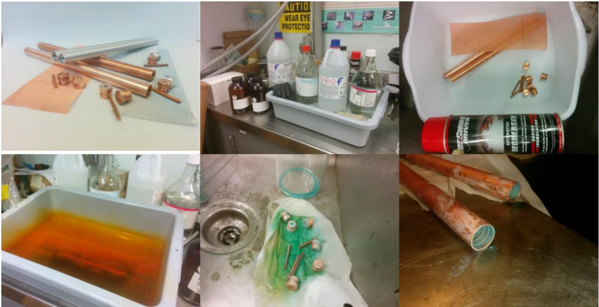
FIGURE 57: THE INITIAL CLEANING PROCESS USING ACID MIXES FOR THE COPPER COMPONENTS.
