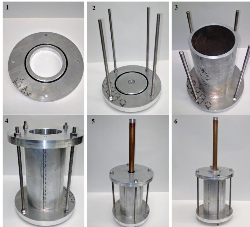
FIGURE 35: THE CONTAINER USED FOR THE HOLDING THE BATH OF ACETONE AND SOLID CO 2 USED AS THE EXPERIMENTAL HEAT SINK. 1. UPPER PLATE. 2. LOWER PLATE WITH HOLE FOR HEAT PIPE AND READY ROD HOLES FOR O-RING COMPRESSION. 3. SAME AS 2. WITH CONTAINER FOR HEAT SINK MATERIALS. 4. ASSEMBLED CONTAINER. 5. AN UPSIDE DOWN VIEW WITH THE HEAT PIPE INSERTED INTO THE BOTTOM AND DISPLAYING THE O-RING THAT WILL BE USED FOR SEALING. 6. COMPLETE ASSEMBLY WITH HEAT PIPE SEALED IN PLACE.
