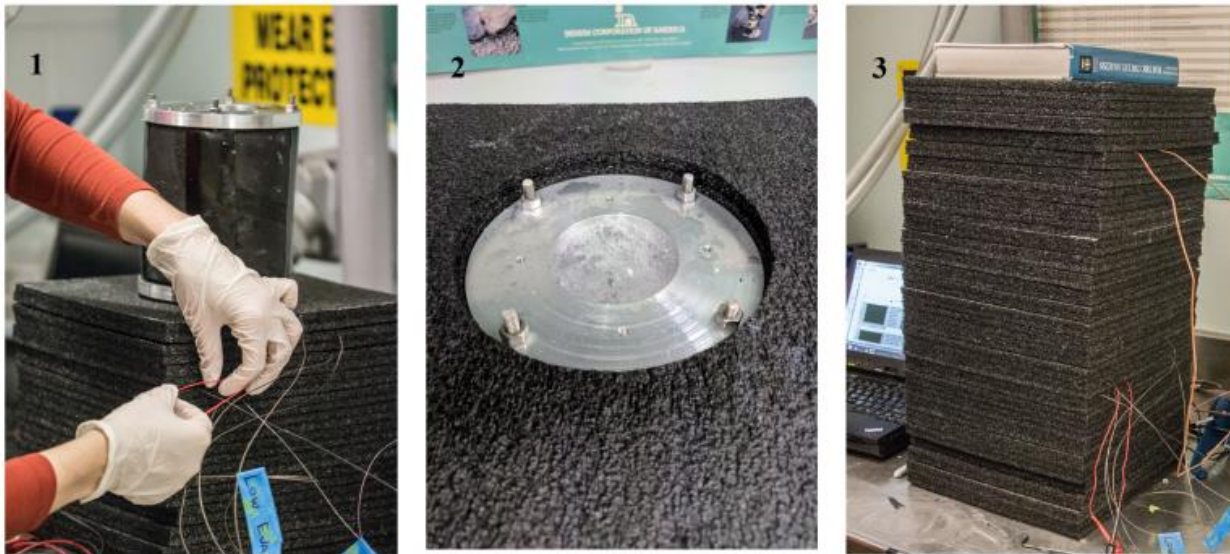
FIGURE 39: PHOTOS OF FINAL EXPERIMENTAL SET UP. PICTURE 2 DISPLAYS THE HEAT SINK FILLED WITH ACETONE AND SOLID \text{CO}_2 .
