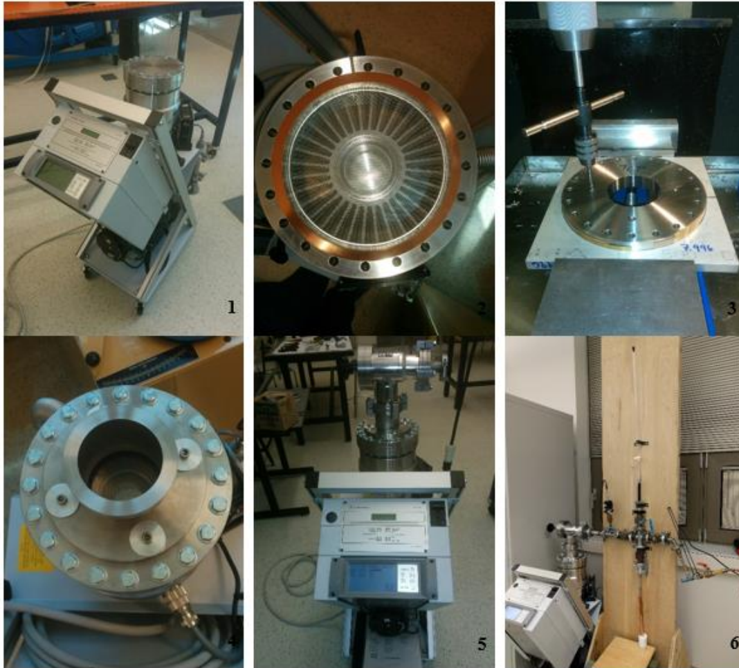
FIGURE 58: PROCESS OF SETTING UP THE EVACUATION AND FILLING RIG. 1. NEW VACUUM PUMP. 2. TOP VIEW OF VACUUM PUMP. 3. MACHINING VACUUM FLANGE. 4. ASSEMBLING VACUUM SYSTEM. 5. ASSEMBLY CONTINUES. 6. COMPLETED EVACUATION AND FILLING RIG.
