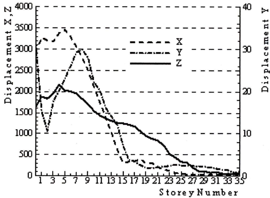
Figure 4.7. Peak displacement of the centerline of model D by SV wave at 60 degree input angle
