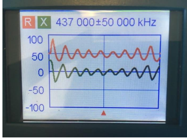
Figure 87: R/X response, \lambda/2 cable, outdoor, antenna analyzer.
