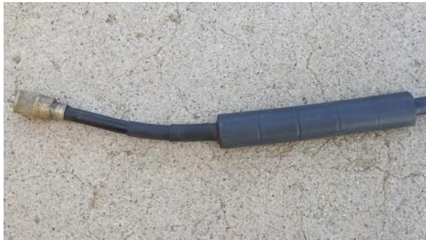
Figure 44: Lossy ferrite choke balun for HF amateur radio. Adapted from [45].
