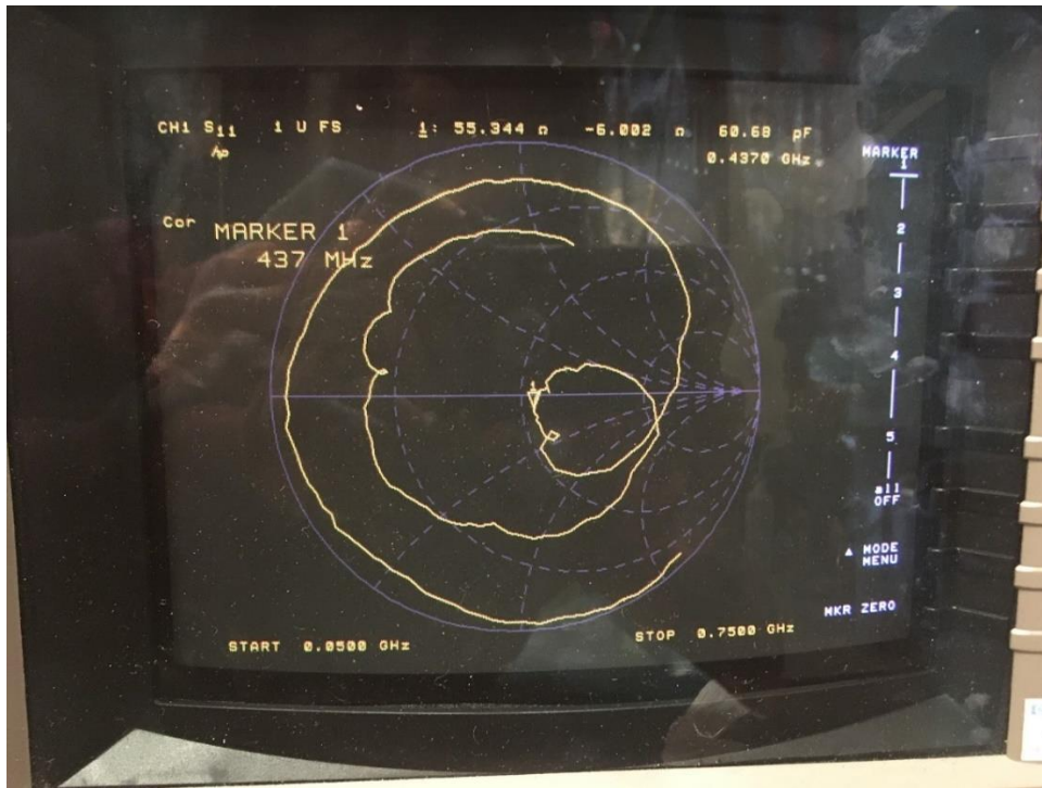
Figure 76: Smith Chart response, \lambda/2 cable, indoor, VNA.
