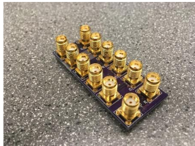
Figure 27: Breakout board for the pre-balun circuit.
