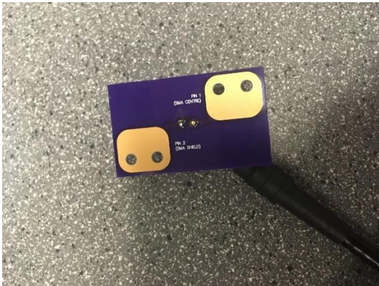
Figure 36: Test PCB, no antenna arms, no GND, test setup.
