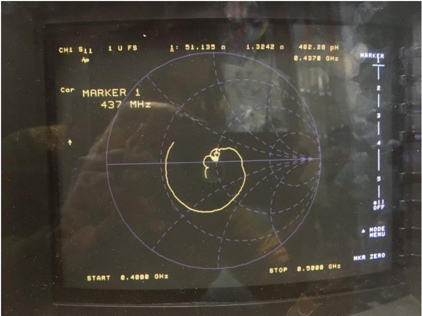
Figure 80: Smith Chart response, extender cable #2, indoor, VNA.
