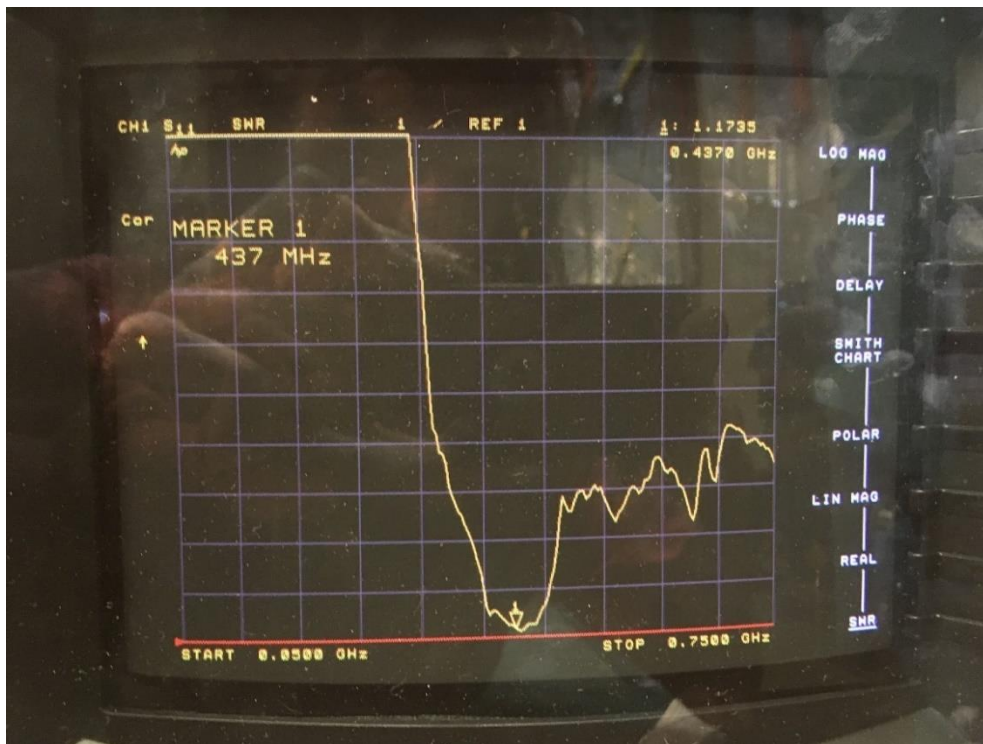
Figure 77: VSWR response, \lambda/2 cable, indoor, VNA.
