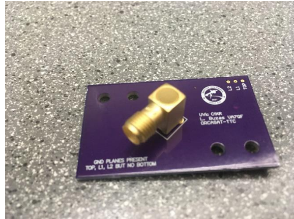
Figure 33: Minimalistic antenna test PCB, connector side.
