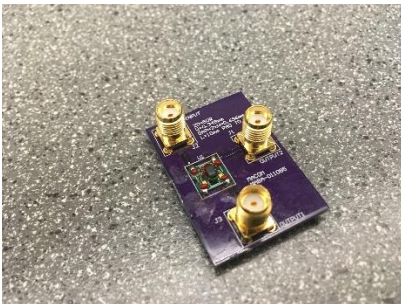
Figure 26: Breakout board for the balun.
