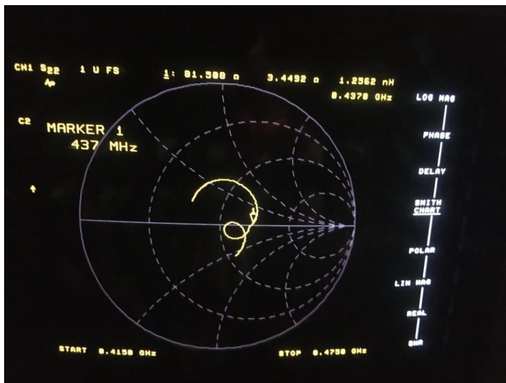
Figure 130: Test antenna Smith Chart captures 437 MHz.
