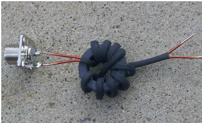
Figure 43: Inductive ferrite choke balun for HF amateur radio. Adapted from [44].
