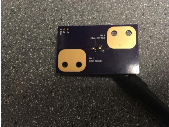
Figure 40: Test PCB with GND, no antenna arms, test setup.
