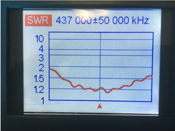
Figure 86: VSWR response, \lambda/2 cable, outdoor, antenna analyzer.
