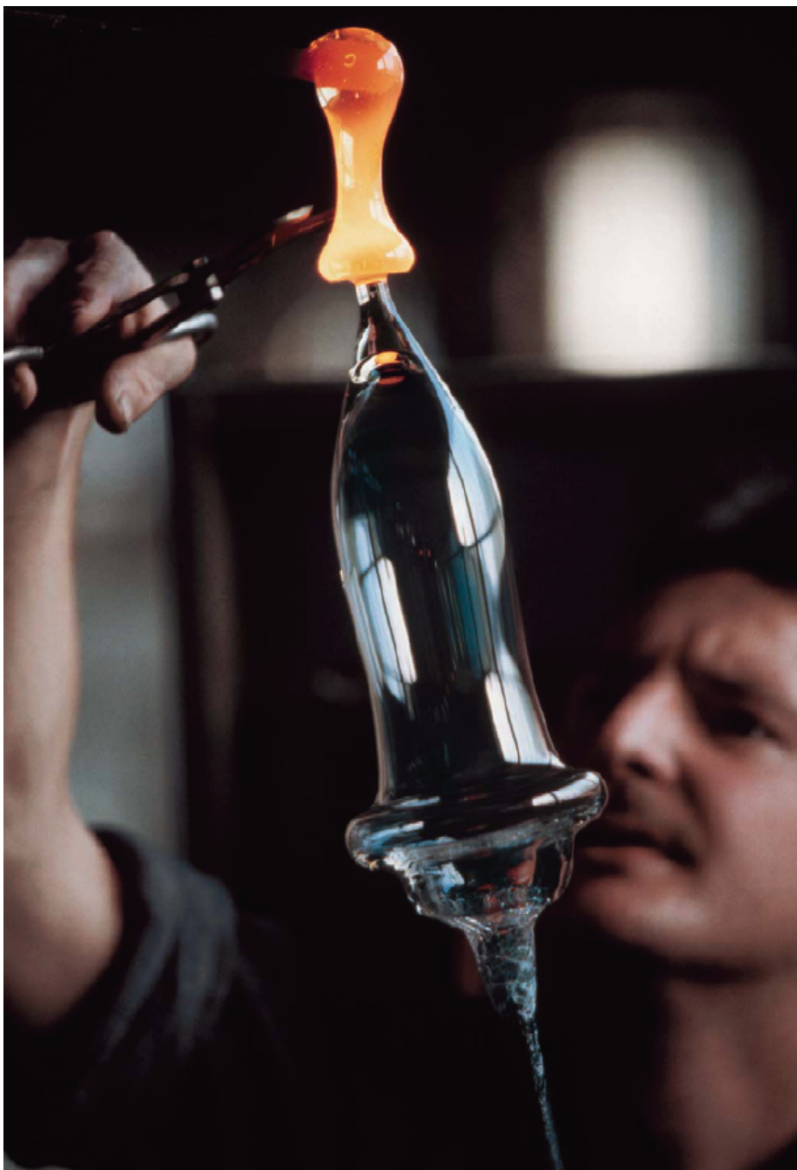
Figure 1.1: A glass tube with air trapped inside heated at one end [4].
