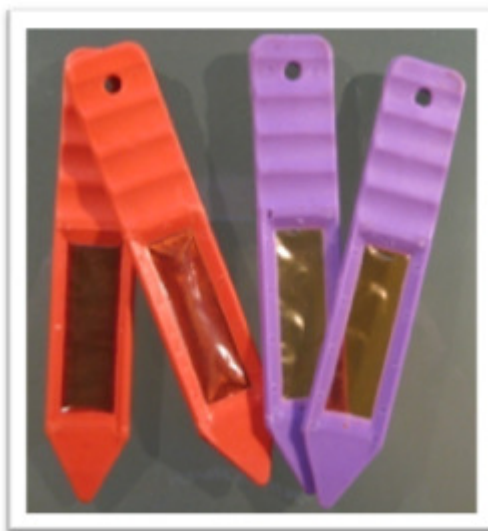
Figure 10 – A PRS™-probe pair consists of one cation (orange) and one anion (purple) probe. Each probe is 15 X 3 cm and has an adsorbing surface area of 17.5 cm 2 (includes both sides).
