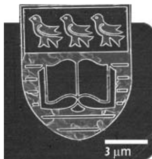
Figure 3.1 Scanning electron micrograph of sub-micron scale crests of the University of Victoria in a Copper TEM grid, fabricated with a Hitachi FB-2100 FIB [ Reproduced with permission from 69 ]
