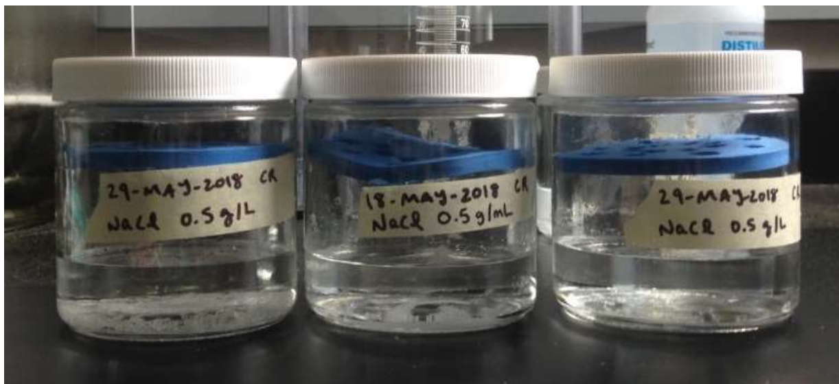
Figure 3-1 Each experimental chamber was prepared with 100 mL of saturated salt solution, a (blue) support (on which the sample was placed), and closed tightly with vacuum grease. A capillary tube of thymol was also placed in each jar to inhibit microbial growth.
