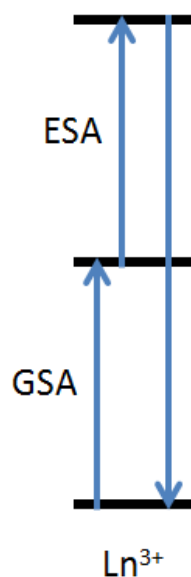
Figure 3.1 —Schematic of the ground state absorption (GSA)/excited state absorption (ESA) mechanism, whereby two successive photons are absorbed, followed by emission of one photon with shorter wavelength (higher energy).
